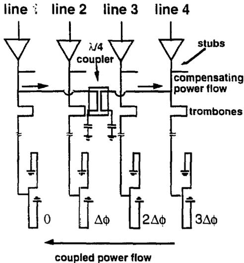
Fig. 4. JET feed circuit schematic.
