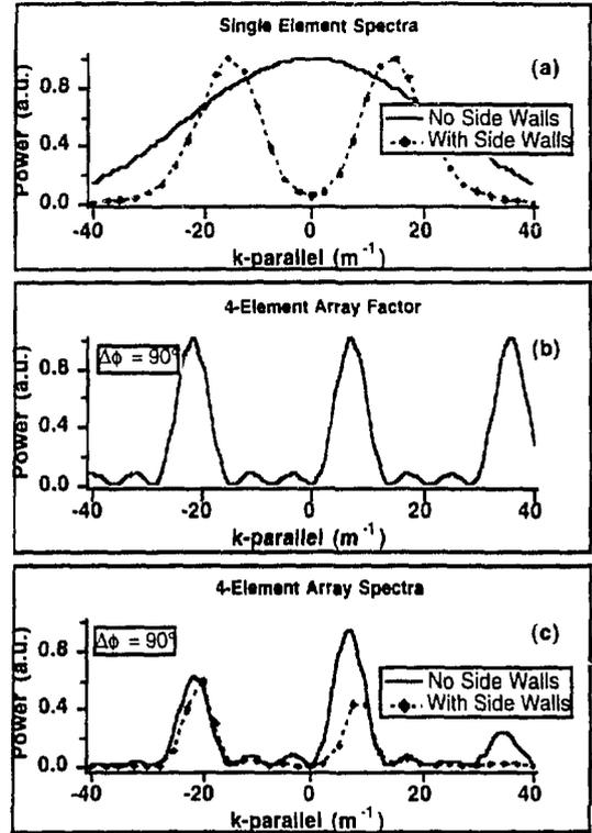
Fig. 2. (a) Single-element spectra for a bare current strap (calculated) and for a strap with side walls (measured on a DIII-D antenna mock-up). (b) The array factor for a four-element array. (c) The resulting spectra for the four-element array with and without side walls.
