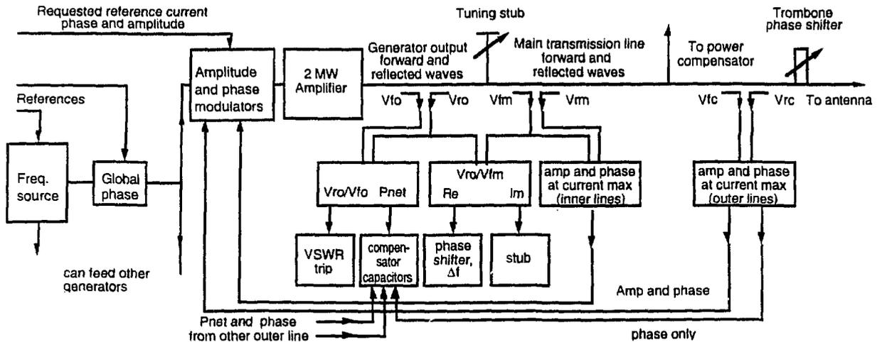
Fig. 6. The JET ICRF automatic control system for feed line 1.
