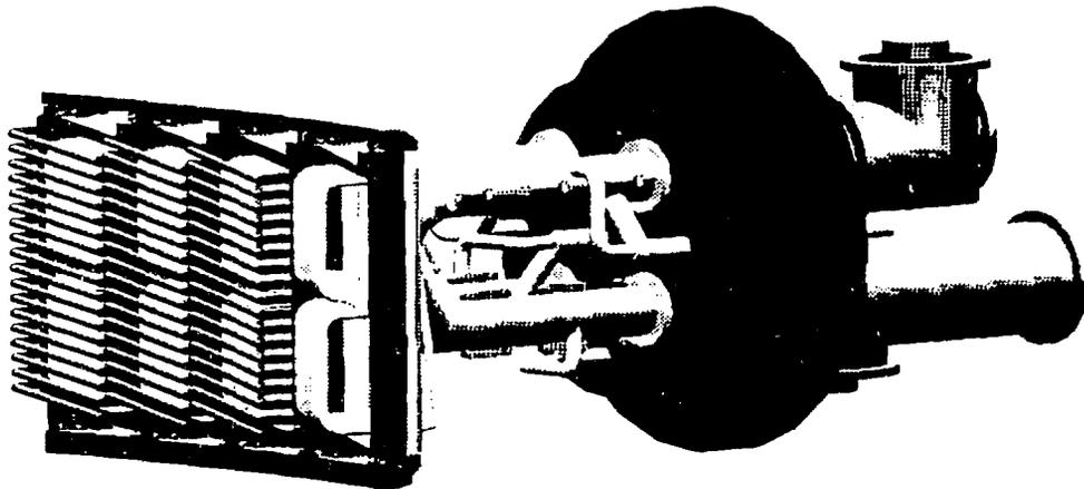
Fig. 1. Conceptual design of a modular four-element FWCD antenna array for DIII-D. This array is designed to operate at 4 MW for pulse lengths of 10 s in the frequency range from 30 to 120 MHz.
