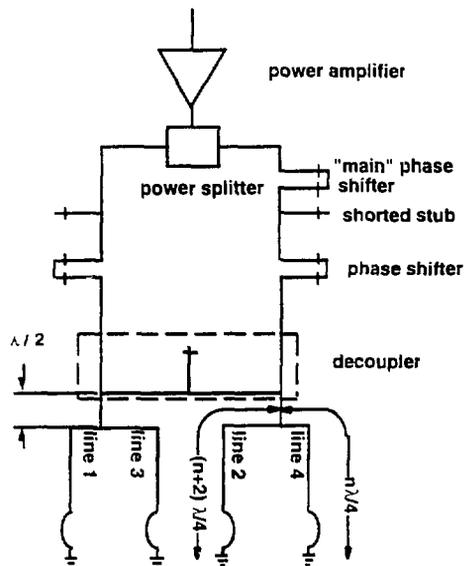
Fig. 5. DIII-D feed circuit schematic.
