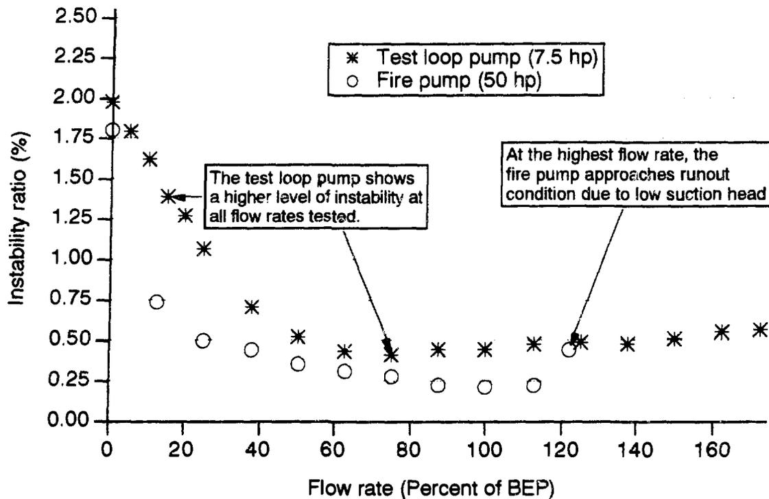
Figure 6. Instability ratio versus flow rate for two pumps
