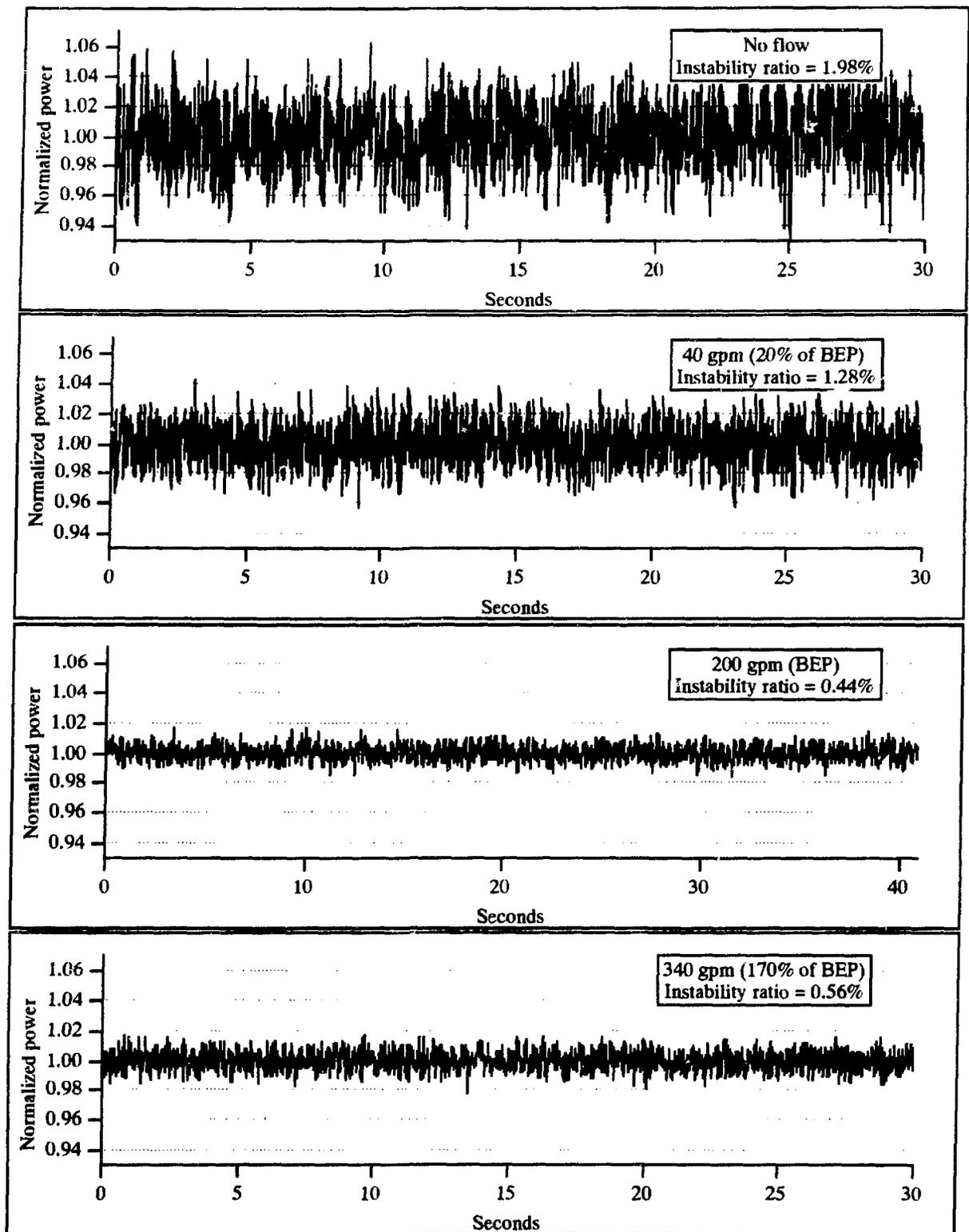
Figure 5. Normalized power at four flow conditions for test loop pump.
