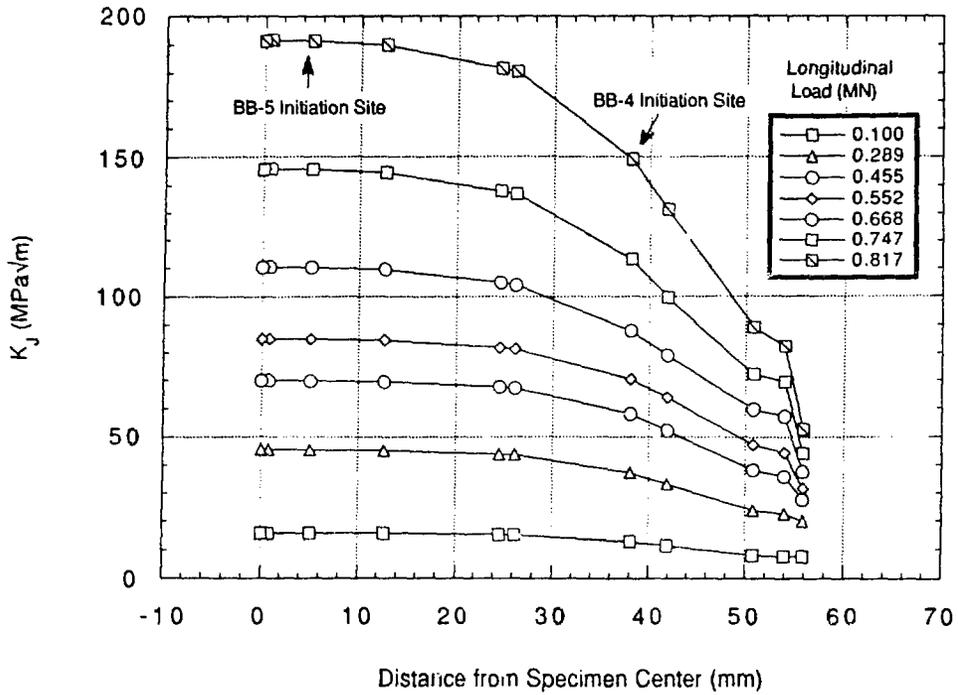
Fig. 14 Variation of  $K_J$  along the crack front for a 0.6:1.0 biaxial loading condition.
