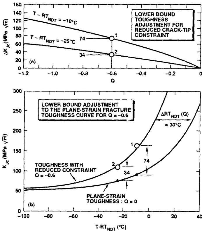
Fig 20. A fracture-toughness curve for a reduced crack-tip constraint condition can be generated using the plane-strain, fracture-toughness curve and the J-Q failure locus envelope.
