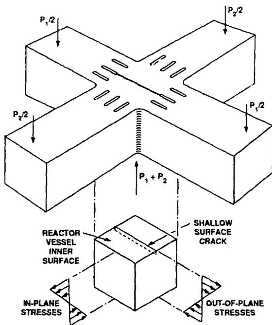
Fig. 8 Conceptual features of the cruciform shallow-flaw, biaxial fracture-toughness test specimen
