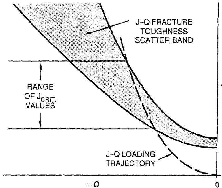
Fig. 3 Intersection of the J-Q loading trajectory for a specific configuration and loading condition with the material J-Q fracture-toughness scatter band defines the range of critical J values
