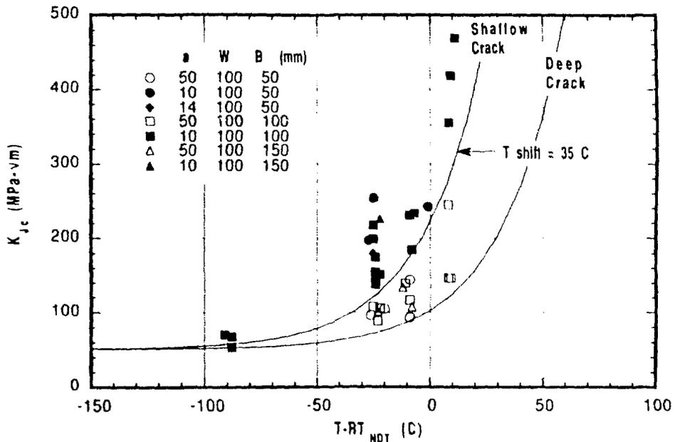
Fig. 5 Data from the shallow-flaw, fracture-toughness testing program show that the shallow-flaw effect produces a substantial increase in toughness at temperatures in the transition region of the fracture-toughness curve.
