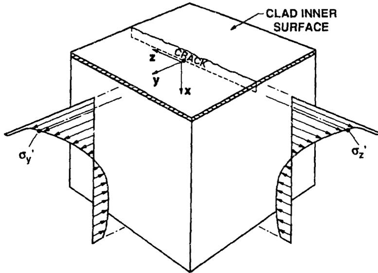
Fig. 7 PTS loading produces biaxial stresses in a reactor vessel wall with one of the principal stresses aligned parallel with the tip of a constant depth shallow-surface flaw.
