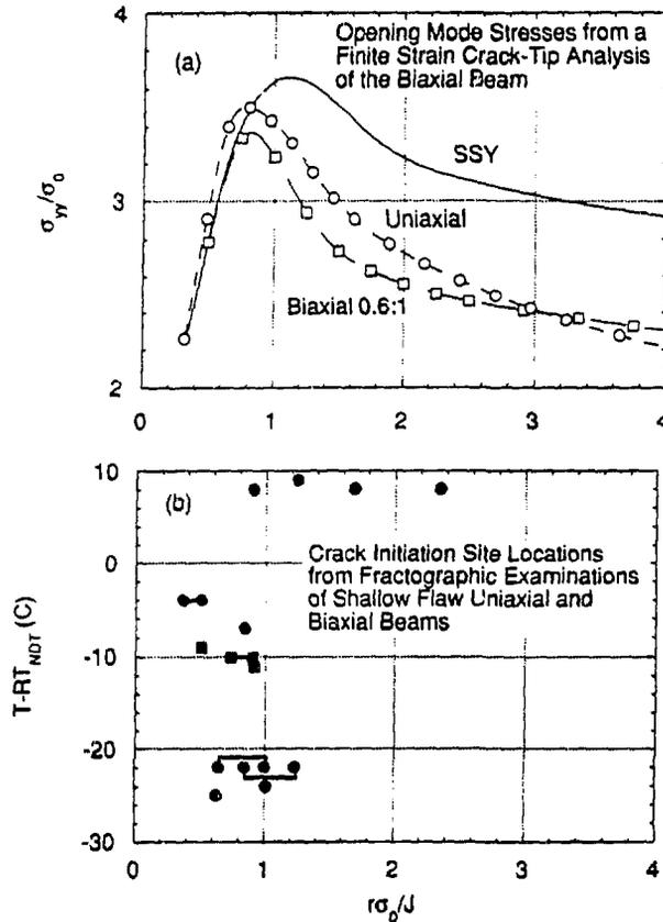
Fig 21. Additional refinement to the crack-tip stress field analysis model appears to be required to reconcile analysis predictions with fractography results.
