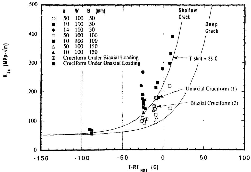
Fig. 18 Biaxial loading resulted in shallow-flaw, fracture-toughness values below the lower bound values obtained under uniaxial loading.
