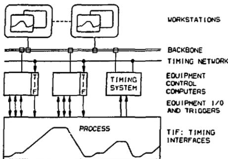
Figure 3: The SIS-ESR Control Architecture
