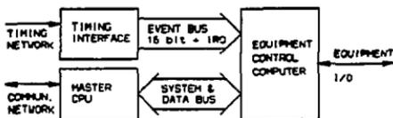
Figure 4: Event-Driven Equipment Control Computer
