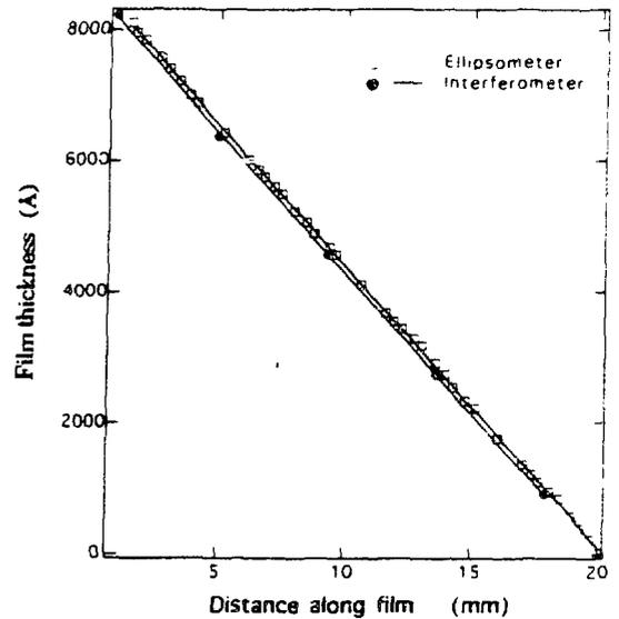
**Figure 4. Experimentally measured film thickness profiles.**
