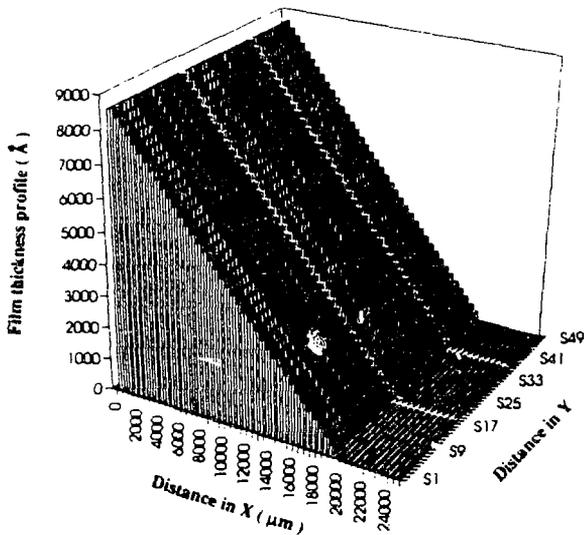
**Figure 5. The 2-D film thickness profile of the standard wedge wafer # 1 measured by Image Scanning Ellipsometer.**
