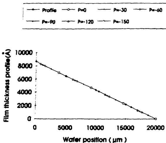
**Figure 1.** Calculated film thickness at the null point versus position for various polarizer settings. System was a particular  $\text{ThF}_4$  solid wedge deposited on a Si wafer.
