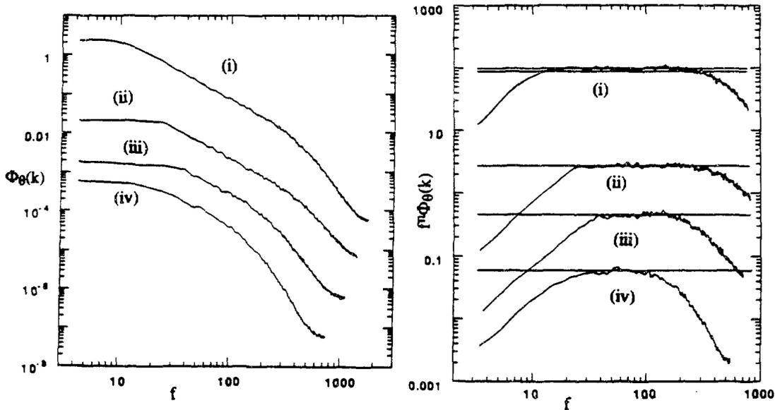
Figure 2 Temperature spectra in grid turbulence with a linear (passive) temperature gradient. a) "Raw" spectra, b) spectra of a) multiplied by  $f^n$  where  $n$  is the slope of the scaling region in a). The Reynolds number for the four spectra are (i)  $Re_l = 856$ , (ii)  $Re_l = 282$ , (iii)  $Re_l = 67$ , (iv)  $Re_l = 59$ .
