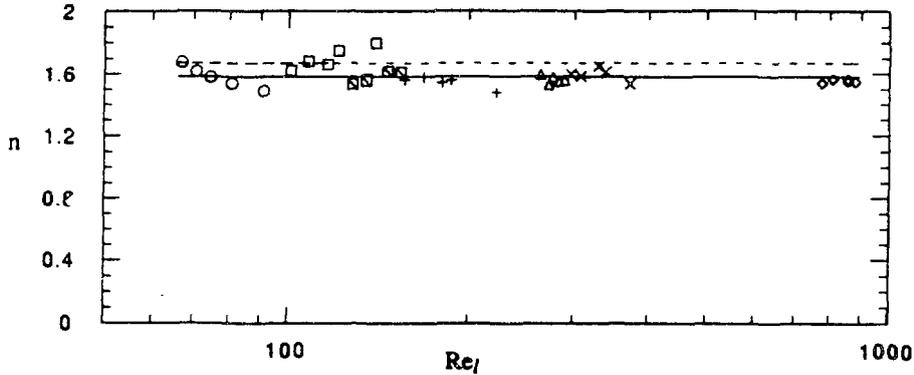
Figure 3. The slope of the scaling region for all experiments as a function of  $Re_l$ . The mean value is 1.58 (solid line). It is within one standard deviation of the Kolmogorov value of  $5/3$ . The  $\blacksquare$  symbols are for no temperature gradient (mandoline), all other symbols are for the toaster.
