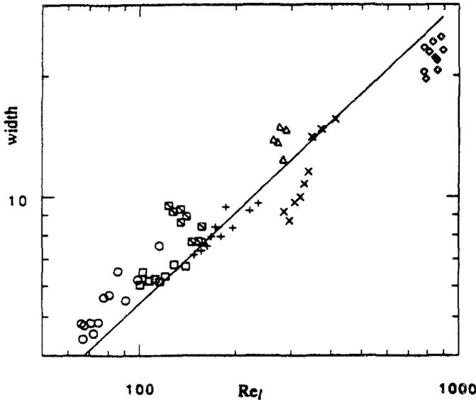
Figure 4. The width of the scaling region as a function of  $Re_l$ . The solid line has a slope of 0.75, the value predicted using Kolmogorov scaling:  $l/\eta \sim Re_l^{0.75}$ .
