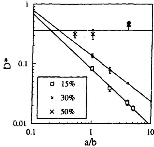
Figure 5: The dimensionless dispersivity as a function of the ratio of the radius of the settling ball ( $a$ ) to the radius of the suspended spheres ( $b$ ) for various volume concentrations of solids: 15 vol% ( $\square$ ), 30 vol% ( $\bullet$ ), or 50 vol% ( $\times$ ). The error limits shown are based on the nonlinear analysis which assumes that the time scale is known exactly, so they represent a minimum for the actual 95% confidence limits.
