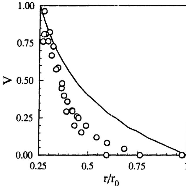
Figure 2: Steady-state velocity profile for a suspension of 50 vol % spheres with a mean diameter of 675  $\mu\text{m}$ . The azimuthal velocity was measured along one diameter of the image. The solid curve is the velocity profile for a Newtonian fluid.
