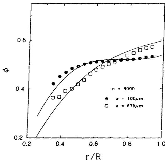
Figure 4: Measurements and predictions of the concentration profiles for suspensions of 50 vol% of either 100  $\mu\text{m}$  (●) or 675  $\mu\text{m}$  (□) particles. Both results are shown for 8000 rotations of the inner cylinder. Model parameters are unchanged from those used in Figure 3.
