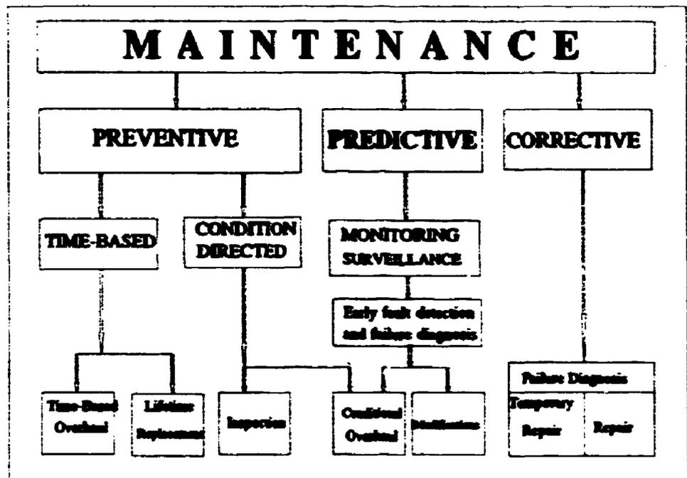
Fig. 4 : Representation of the role of monitoring in NPP maintenance
