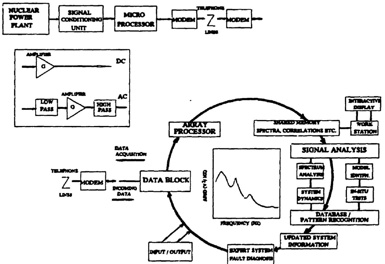
Fig. 2: Data acquisition and on-line signal analysis system
