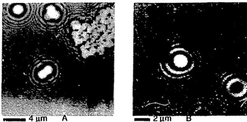
Fig. 6. (a) hologram of 1.09 μm-diameter latex spheres recorded on PMMA with 1.89 nm x-rays and read out on a 512x512 grid of 40nm pixels using the AFM, (b) similar hologram of 30 nm-diameter gold spheres read on a 600x600 grid of 25nm pixels.
