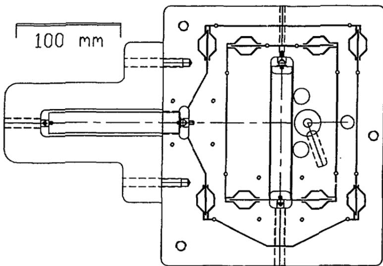
Fig. 3. Mechanical layout of the x - y scanning stage of the atomic force microscope
