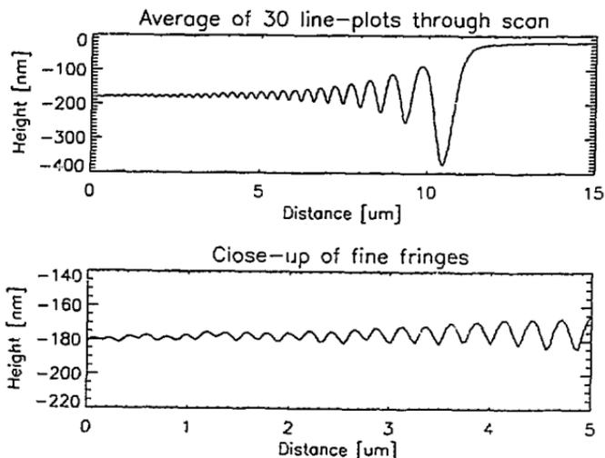
Figure 8. Overviews and close-ups of the hologram of a 12  $\mu\text{m}$ -diameter gold wire recorded on PMMA with 1.89 nm x-rays. The left-hand hologram is read on a 400x400 grid of 150nm pixels and the right hand one on a 512x512 grid of 40nm pixels. The graphs are made by integrating the two-dimensional data over the rectangular area marked on the right hand hologram. The smallest recorded oscillations have an amplitude of 2-3nm.
