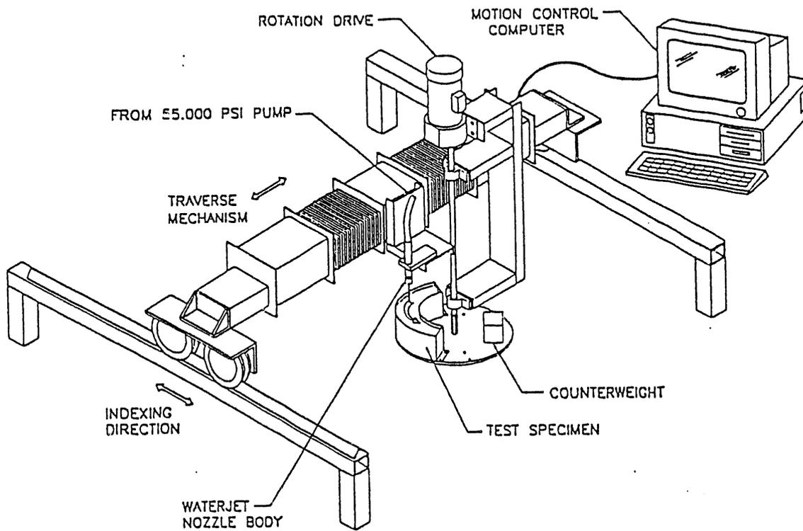
**Figure 2. Scarifier Separate Effects Experiment Test Fixture**
