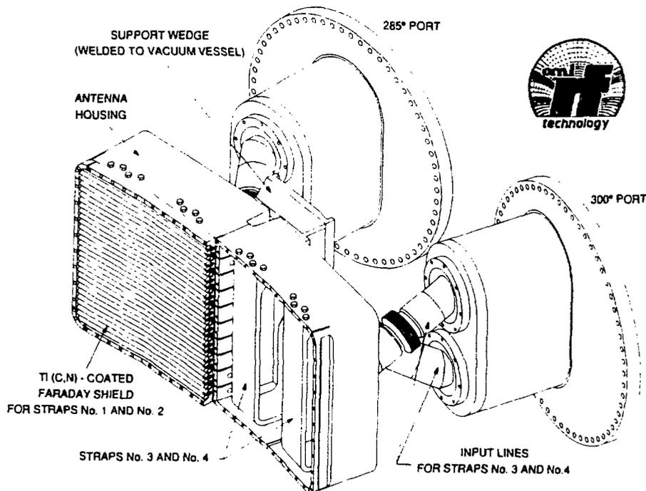
Fig. 1. Fast wave current drive antenna for DIII-D (30-60 MHz, 2 MW, 2 s, four strap)
