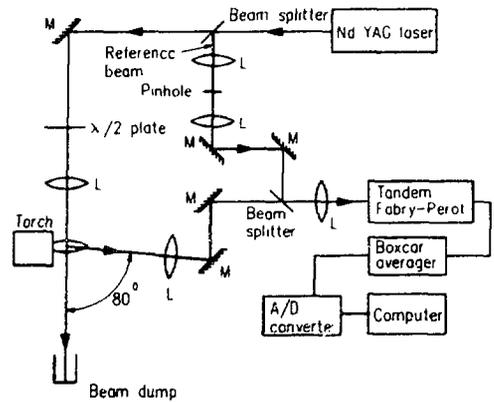
Figure 4. Experimental setup to measure the ion feature.
