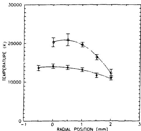
Figure 7. Radial temperature profiles of a free-burning arc at 2 mm below the cathode. The solid dots are the gas temperature. The open circles are the electron temperature.
