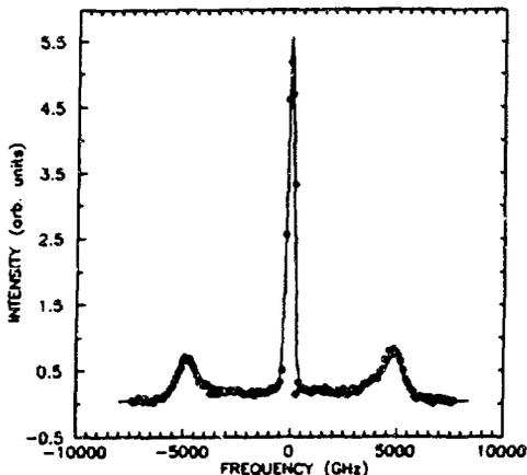
Figure 5. Electron feature in a free-burning arc at 2 mm below the cathode at the radial position  $r \approx 0$  mm.  $T_e = 28240$  K  $\pm$  3% and  $n_e = 1.62 \times 10^{23}$  m $^{-3}$   $\pm$  3%.
