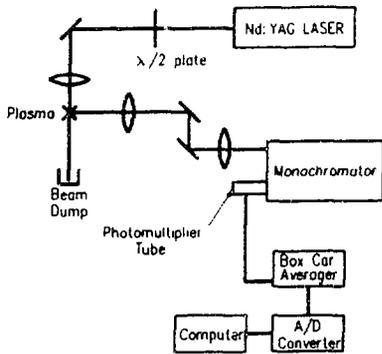
Figure 3. Experimental setup to measure the electron feature.
