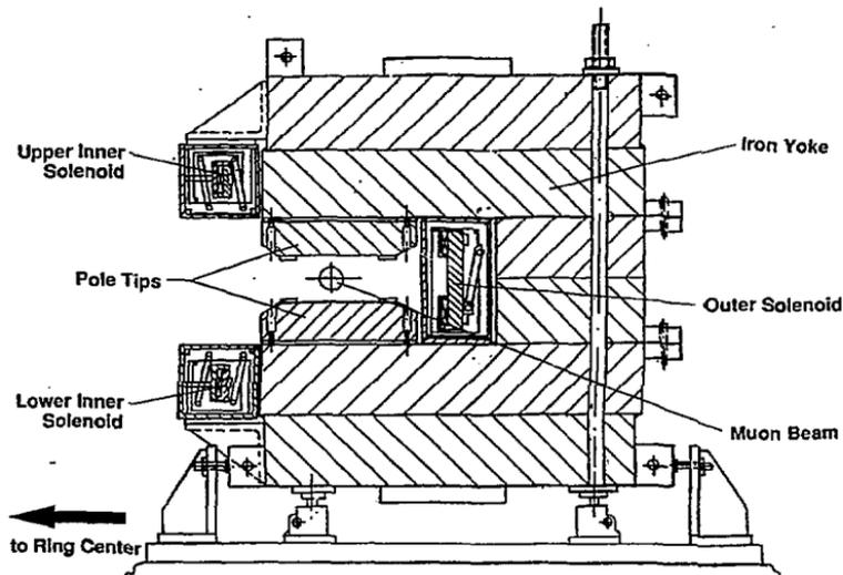
Fig. 1 A Cross-section view of the g-2 storage ring showing the three large solenoids
