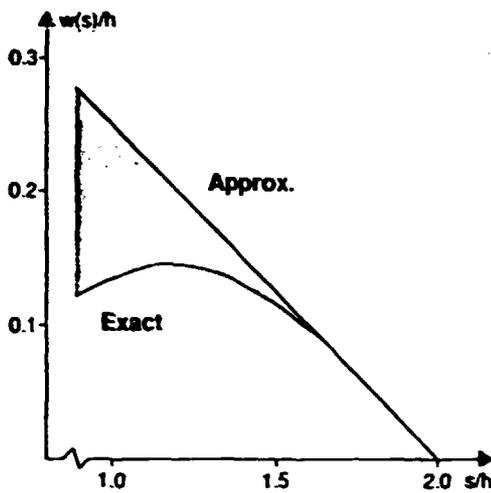
Figure 7 Validity of the linear approximation of the exposure width.  $\theta=30^\circ$  and  $c=0$
