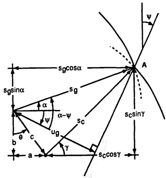
Figure 3 Ground wire shielding effect analysis
