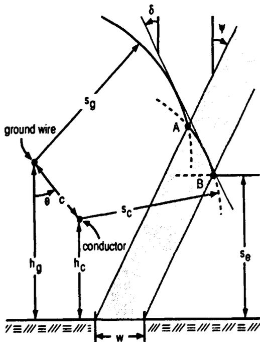
Figure 1 Definition of exposure width
