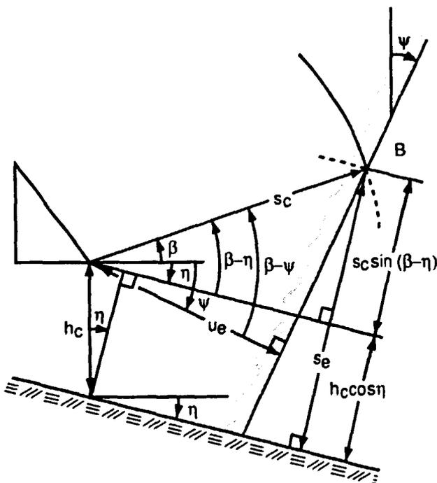
Figure 4 Earth surface shielding effect analysis
