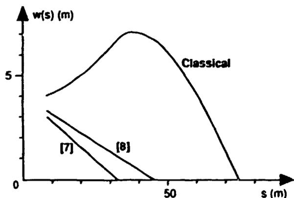
Figure 8 Comparison of exposure width functions.  $\theta=30^\circ$ ,  $c=8$  m, and  $h_{am}=37.5$  m
