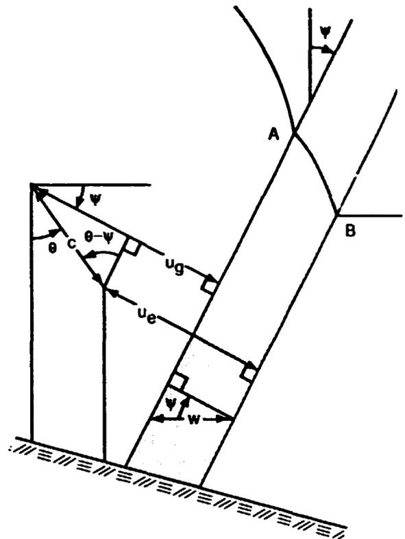
Figure 2 Decomposition of exposure zone width
