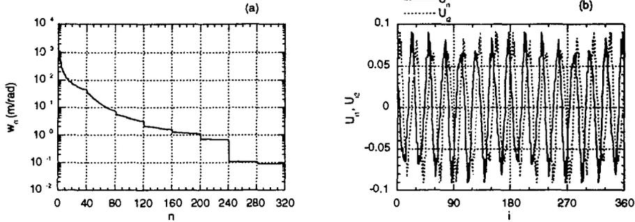
Fig. 3: (a) Plot of the eigenvalues in descending order for the APS storage ring with  $M = 360$  and  $N = 320$  in the vertical plane and (b) the BPM basis vectors  $U_{i1}$  and  $U_{i2}$  ( $1 \leq i \leq 360$ ) for the most strongly coupled channels.
