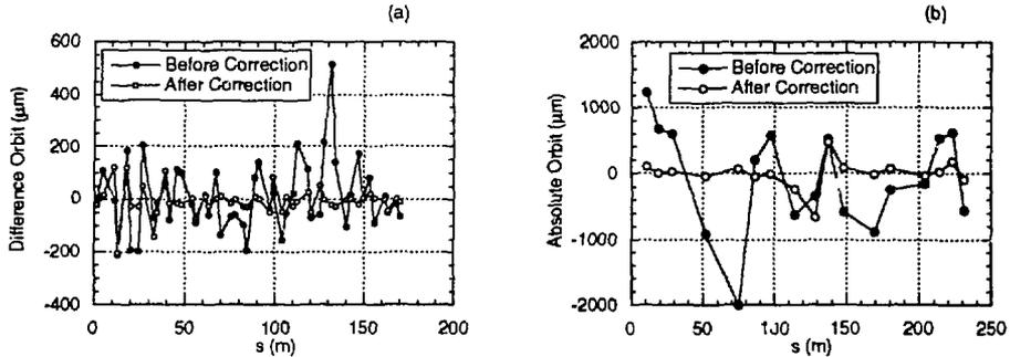
Fig. 1: DC global orbit correction on (a) the NLSL X-ray ring and (b) SPEAR, SSRL.
