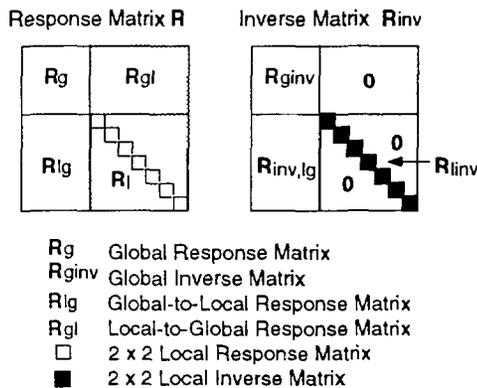
Fig. 6: Response matrix and its inverse for the unified feedback system.
