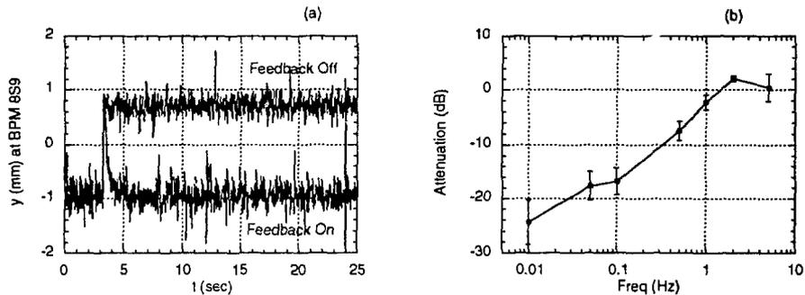
Fig. 2: Result of global orbit feedback on SPEAR, SSRL in (a) time domain and (b) frequency domain. The parameters used were:  $K_p = 3$ ,  $K_I = 0.05$ ,  $K_D = 0$ ,  $F_s = 37$  Hz, and  $f_b = 0.37$  Hz.
