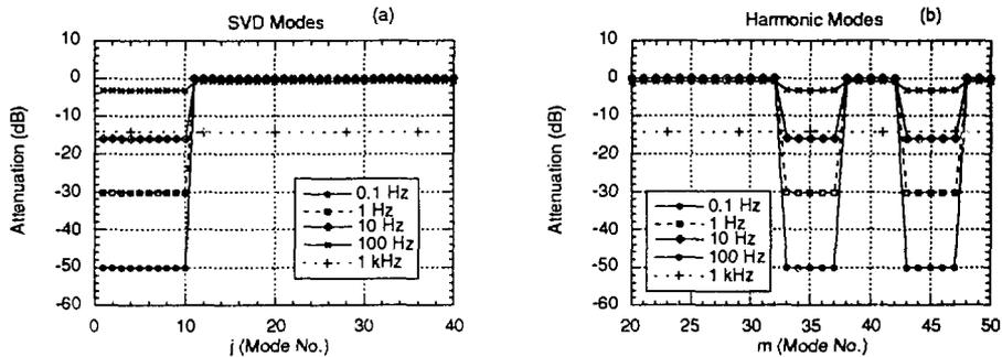
Fig. 4: Correspondence between the (a) SVD eigenmodes and (b) harmonic modes for global AC feedback in the horizontal plane of the APS storage ring. The ten largest SVD eigenvalues are used for orbit correction in the horizontal plane.
