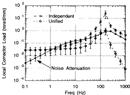
Fig. 7: Improvement of local orbit correction efficiency for the unified system. The noise sources are SVD eigenmodes. Random field error less than 2% and orbit deviation less than 3 mm were assumed with the vacuum chamber eddy current taken into account.
