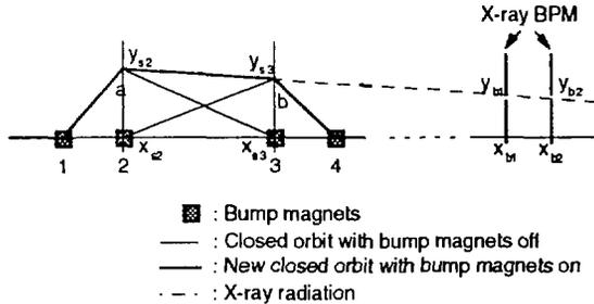
Fig. 5: Four-magnet bump to control the position and the angle of the X-ray radiation, which comprises two three-magnet bumps a (magnets 1, 2, and 3) and b (magnets 2, 3, and 4).
