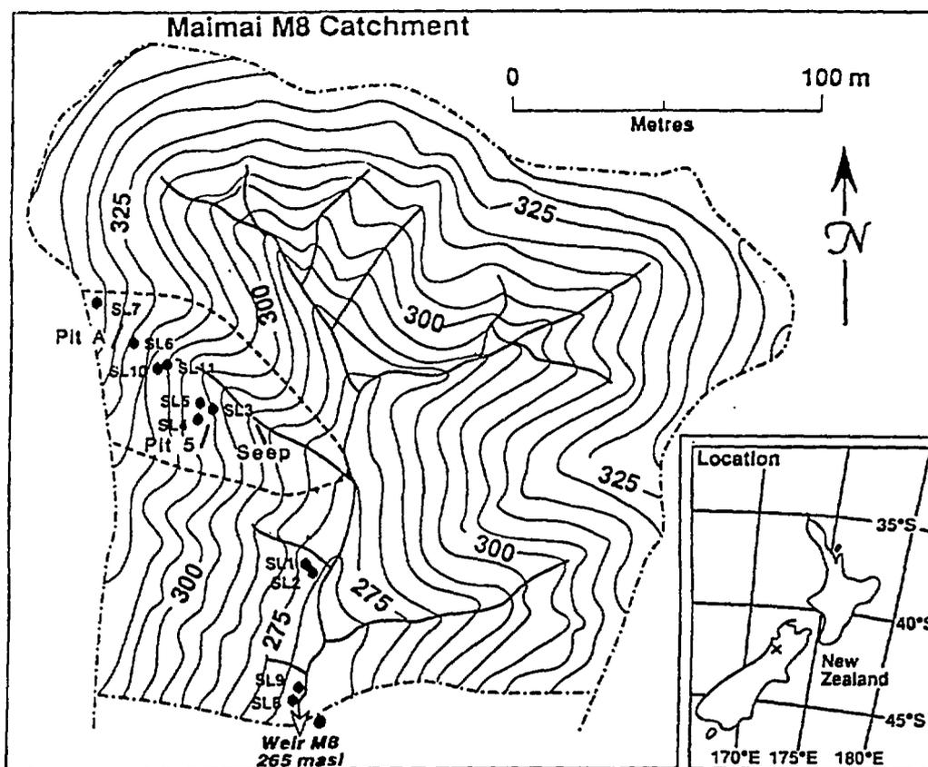
Fig. 1. Maimai 8 catchment showing suction lysimeter (SL) and pit locations.
