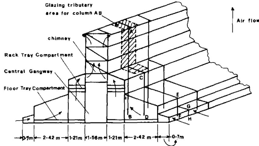
FIGURE 1 Schematic Illustration of the Solar Rice Dryer.
