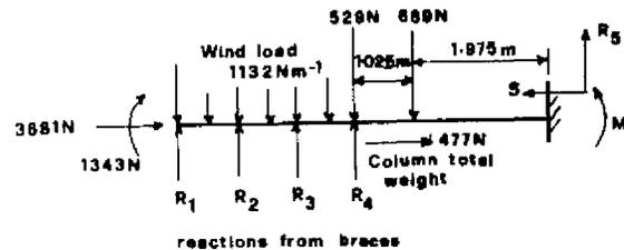
FIGURE 3 A Simplified Loading Diagram for the Main Column.
