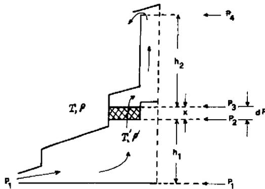
FIGURE 2 Illustration of Pressure Differences within the Solar Dryer Chamber.
