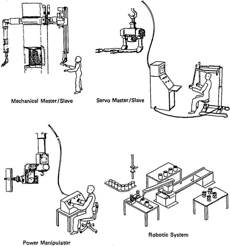
Fig. 1. Four types of manipulators.
