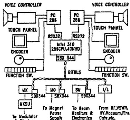
Fig.1 I&C architecture for Preinjector of PLS
