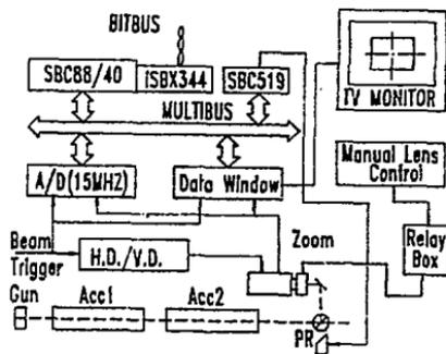
Fig.2 Beam Station Schematic
