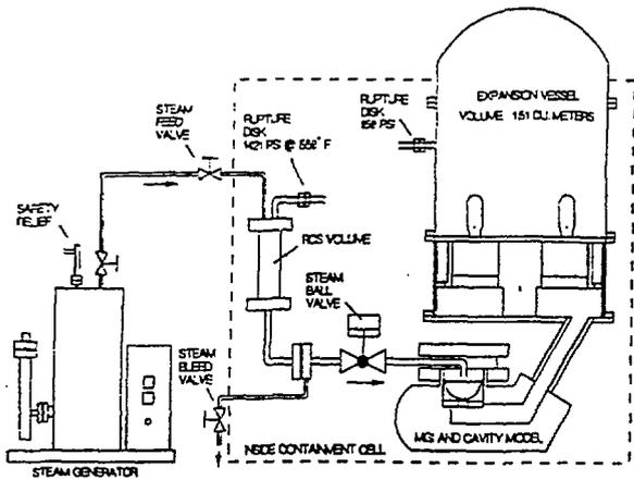
Figure 1 The COREXIT Facility
