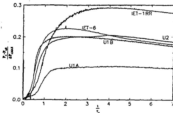
Figure 7 Containment Pressure History Plotted as an Efficiency
