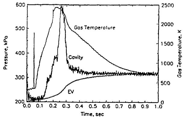
Figure 5 Cavity Pressure and Gas Temperature in DCH-U1B
