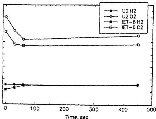
9 Number of Hydrogen and Oxygen Moles in the Containment in the Hydrogen Combustion Tests
