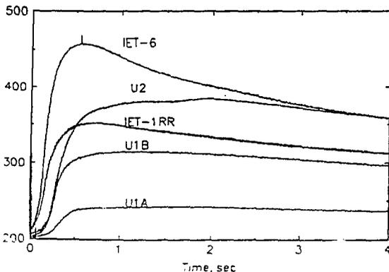
Figure 6 Containment Pressure Histories Obtained in the Experiment
