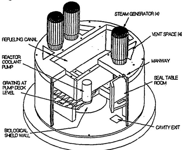
Figure 2 The 1/40 Scale Zion Subcompartment Model
