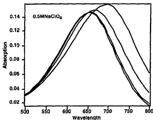
Figure 19. The spectra of the benzophenone anion in 0.5 M NaClO<sub>4</sub> in acetonitrile at 2 ns, 5 ns, 10 ns, and 15 ns after formation. The spectra show a blue shift as a function of time.
