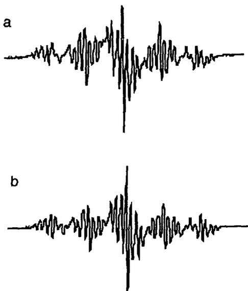
Figure 1. (a) EPR spectrum observed at 100 K after 77 K irradiation of 2% 1,4-cyclohexadiene adsorbed on Na-ZSM-5. (b) EPR spectrum observed at 90 K after 77 K irradiation of 1.5% 1,3-cyclohexadiene adsorbed on Na-ZSM-5.
