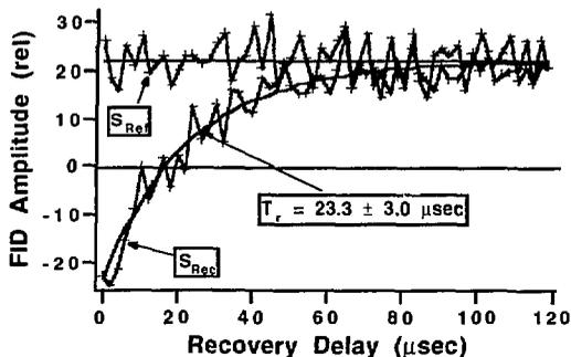
Figure 15. Dynamic inversion recovery of the H atom high-field line, in ice at  $-6^\circ\text{C}$ . On alternating radiolysis shots, a  $70 \text{ ns}$  microwave inversion pulse was applied to produce the "recovery" signal  $S_{\text{rec}}$ . This experiment is performed on the very small signal remaining some  $2.8 \text{ ms}$  after a  $400 \text{ rad}$  radiolysis pulse. The true "zero" level is inferred from half the initial difference in  $S_{\text{ref}} - S_{\text{rec}}$ .
