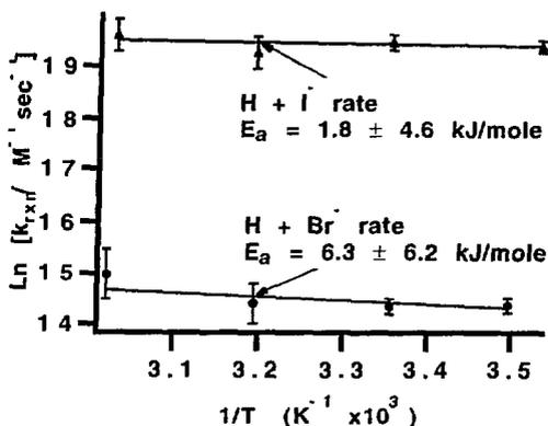
Figure 12. Arrhenius plots of  $\text{Ln}[k_{\text{rxn}}]$  vs.  $1/T$  for the reaction of H atoms with  $\text{I}^-$  and  $\text{Br}^-$  in aqueous solution.
