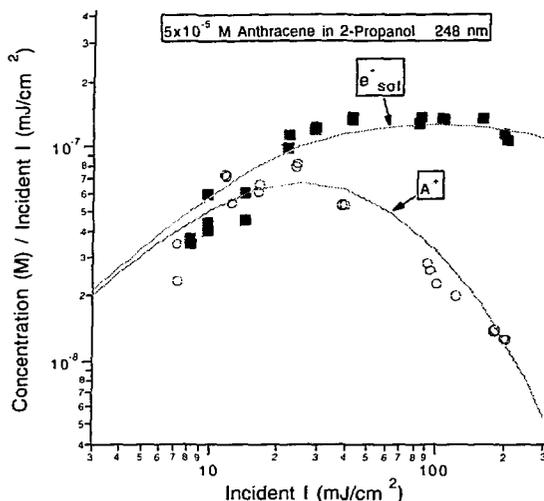
Figure 8. Intensity dependence of ionization in  $5 \times 10^{-5}$  M anthracene in 2-propanol at 248 nm. The upper set of points is for a solution degassed by bubbling with argon, and the lower set with  $\text{SF}_6$ . The concentrations were obtained from the  $e_{\text{sol}}^-$  absorption at 840 nm and the anthracene radical cation absorption at 720 nm for the upper and lower sets, respectively. The curves are calculated as described in the text.
