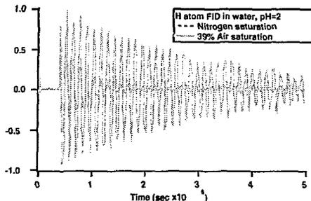
Figure 9. Typical FIDs of the H-atom low-field ( $m_l = +1/2$ ) line immediately following pulse radiolysis of pH 2 aqueous solution. The FID is attenuated in the partially air-saturated solution by the presence of O<sub>2</sub>.
