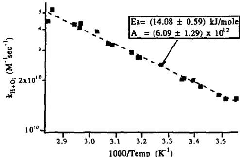
Figure 10. Rate constants for bimolecular dephasing of H atoms by O<sub>2</sub> in H<sub>2</sub>O.
