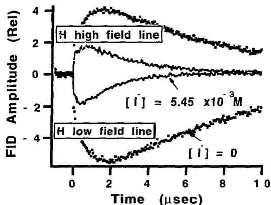
Figure 13. Effect of  $\text{I}^-$  on H-atom CIDEP in pH 3 perchloric acid solution at  $25^\circ\text{C}$  following a 25 ns radiolysis pulse. In the presence of  $5.45 \times 10^{-3} \text{ M}$  iodide, the chemical lifetime of the H atoms should be only 680 ns, but magnetization persists beyond  $10 \mu\text{s}$ .
