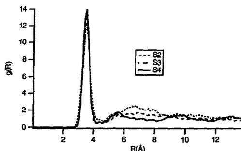
Figure 23. The radial distribution function  $g(R)$  as a function of distance  $R$  (in angstroms).  $R$  is measured from the central ion to the center of the dipole. S2, S3, and S4 are solvent molecules of length two, three, and four elements, respectively.
