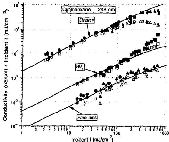
Figure 5. Intensity dependence of ionization in cyclohexane at 248 nm. The upper set of points is for a solution degassed by bubbling with argon, and the middle and lower sets with  $\text{SF}_6$ . The various symbols represent different conditions of laser operation or treatment of the data. The curves are calculated as described in the text, for a two-photon ionization process.
