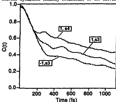
Figure 25. The solvation correlation function as a function of time for solvent molecules of three and four elements and as a function of the charge of the central ion.
