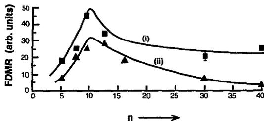
Figure 4. Dependence of the FDMR amplitude in micellar solutions on the number of oxyethylene units,  $n$ , in Triton X detergent molecules in (i) aqueous and (ii) 2-propanol solutions (at  $-10$  K).
