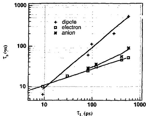
Figure 18. Solvation time of the benzophenone anion, the electron, and a dipole versus the longitudinal relaxation time of the solvent,  $\tau_L$ .
