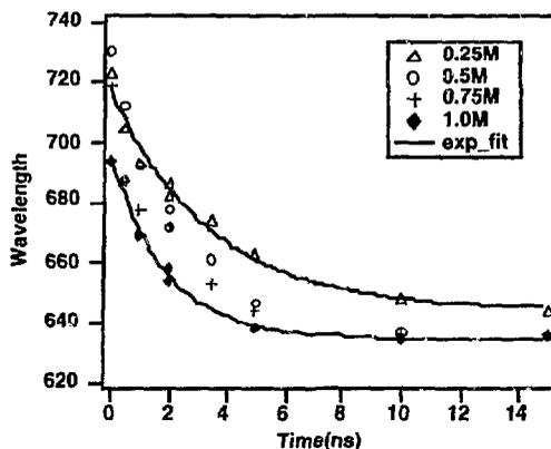
Figure 20. The peak of the absorption spectrum of the benzophenone anion vs. time for four different concentrations of NaClO<sub>4</sub> in acetonitrile.
