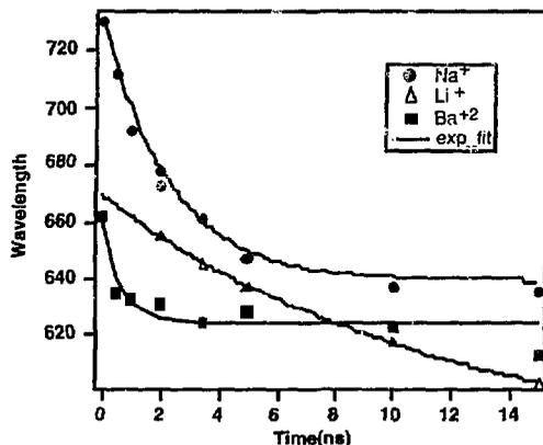
Figure 21. The peak of the absorption spectrum of the benzophenone anion vs. time for 0.5 M NaClO<sub>4</sub>, LiClO<sub>4</sub>, and BaClO<sub>4</sub> in acetonitrile.
