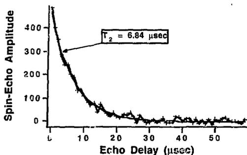
Figure 16. Spin-echo decay envelope of the H-atom high-field line in  $-6\text{ }^{\circ}\text{C}$  ice at  $50\ \mu\text{s}$  following pulse radiolysis with ca. 700 rad radiation pulses. An average of nine similar curves at different time delays and on different days gave  $6.9 \pm 1.0$  for our best estimate of  $T_2$ .
