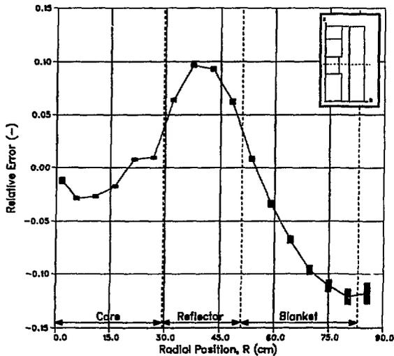
Fig. 2a. Relative Error in Group 3 Neutron Flux Versus  $R$  at Axial Coarse Mesh # 12.
