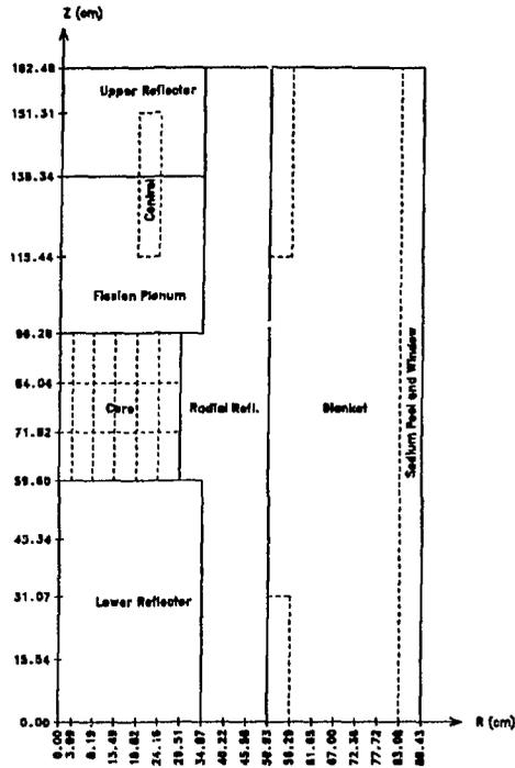
Fig. 1. R-Z Model of EBR-II Showing the Main Regions.
