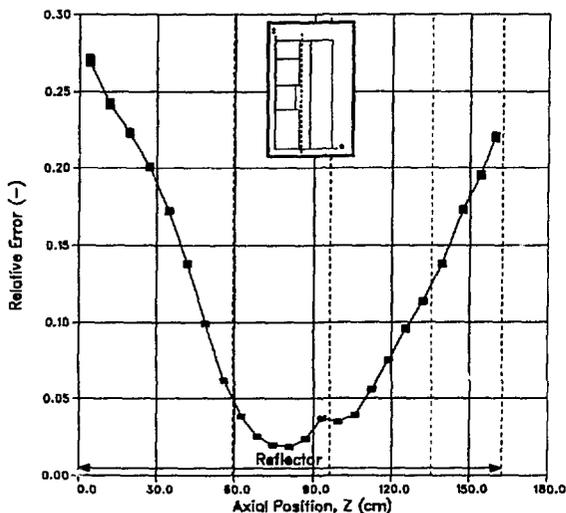
**Fig. 3a. Relative Error in Neutron Heating Versus Z at Radial Coarse Mesh # 8 (Reflector).**
