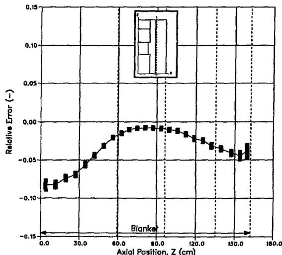
**Fig. 3b. Relative Error in Neutron Heating Versus Z at Radial Coarse Mesh # 11 (Blanket).**
