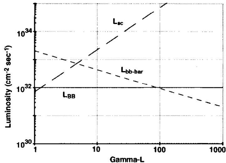
Fig. 1 Luminosity limits due to space charge and beam-beam forces plotted versus the required luminosity for  $b\bar{b}$  events. Beam-beam limits dominate requiring  $\gamma_L > 100$  for sufficient luminosity.
