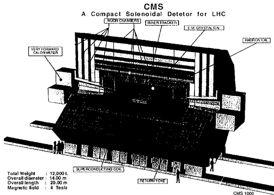
Figure 12. The proposed CMS detector for LHC.
