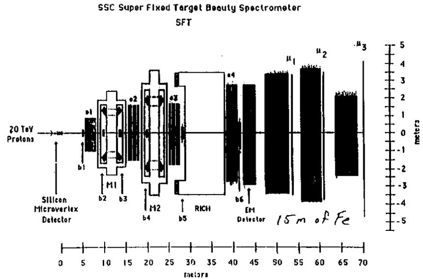
Figure 2. Layout of the proposed SFT spectrometer.
