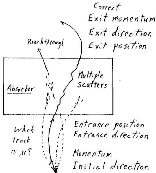
Figure 1. How to identify muons.
