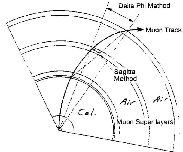
Figure 11. Level 1 muon trigger concept for GEM.
