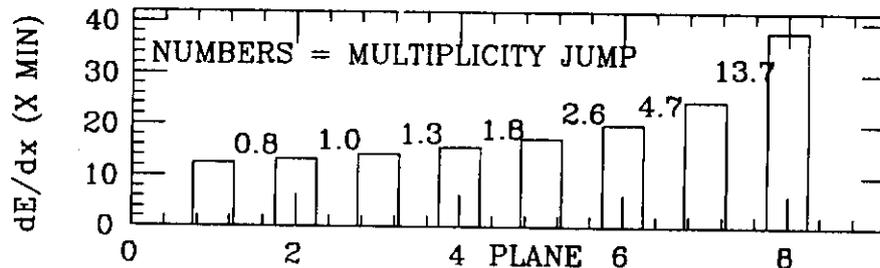
Fig. 4  $dE/dx$  of a stopping proton in 300  $\mu\text{m}$  Si planes expressed as multiples of minimum ionization. Numbers give multiplicity jump between planes.
