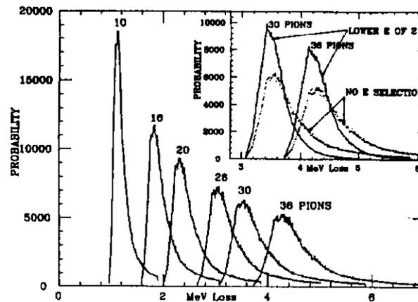
Fig. 2 Some energy loss distributions in 300  $\mu\text{m}$  Si wafers.
