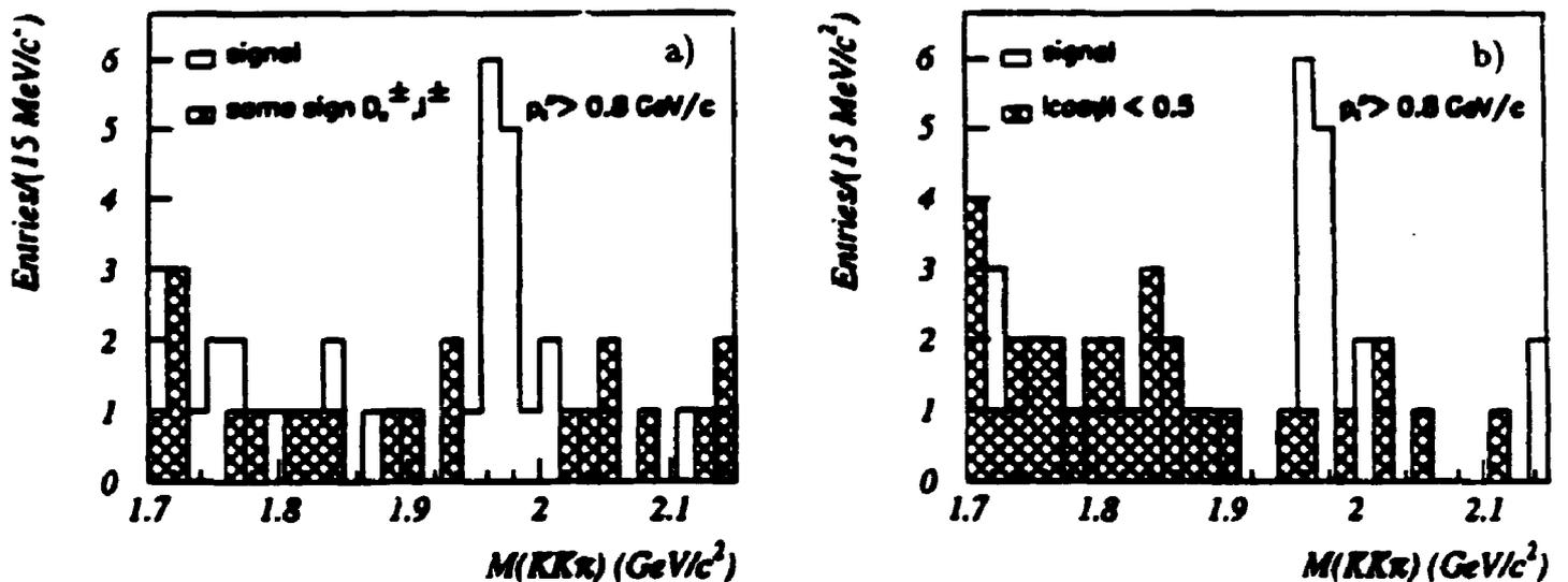
Figure 6: The invariant mass of  $K^+, K^-\pi$  showing a  $D_s$  signal by DELPHI, (a) for opposite sign and same sign (hatched) ( $D_s, \text{lepton}$ ) combinations, and (b) for events accepted and rejected (hatched) by the opening angle cut.
