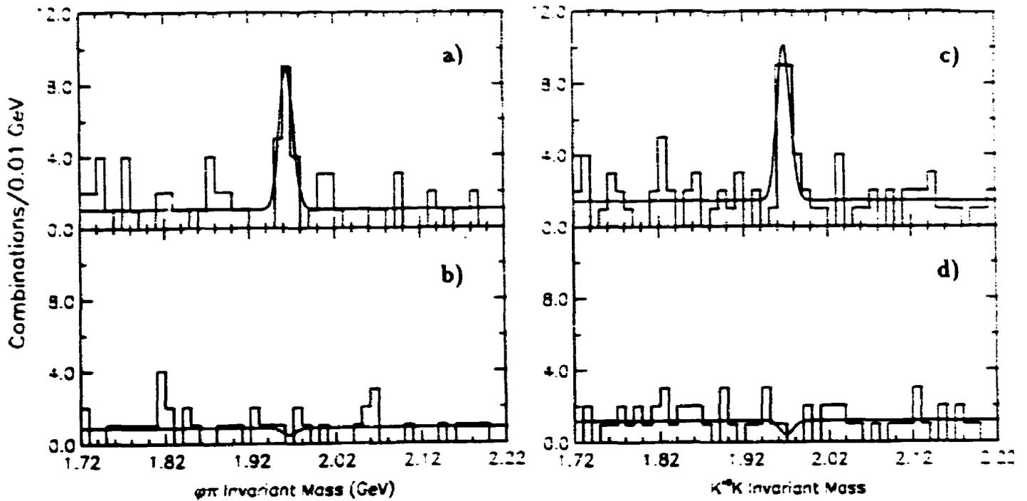
Figure 5: The invariant mass of  $\Phi, \pi$  and  $K, K^0$  showing a  $D_s$  signal for (a) opposite, and (b) same sign ( $D_s, \text{lepton}$ ) combinations by ALEPH.
