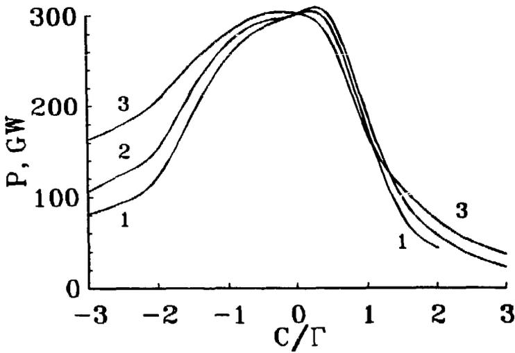
Figure 9: Output FEL amplifier power versus detuning: (1) -  $2 \times 0.25$  TeV variant; (2) -  $2 \times 0.5$  TeV variant; (3) -  $2 \times 1$  TeV variant
