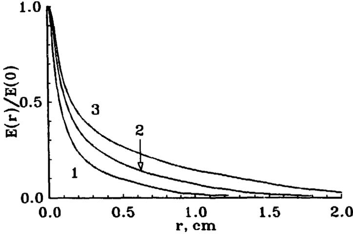
Figure 8: Radiation field distribution versus radius at the FEL amplifier exit: (1) -  $2 \times 0.25$  TeV variant; (2) -  $2 \times 0.5$  TeV variant; (3) -  $2 \times 1$  TeV variant
