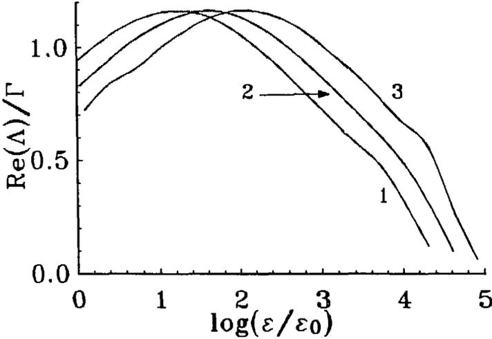
Figure 4: Dependency of the FEL amplifier increment on emittance ( $\epsilon_0 = 10^{-6} \text{ cm} \times \text{rad}$ ): (1) -  $2 \times 0.25 \text{ TeV}$  variant; (2) -  $2 \times 0.5 \text{ TeV}$  variant; (3) -  $2 \times 1 \text{ TeV}$  variant
