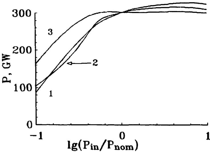
Figure 10: Output FEL amplifier power versus input power: (1) -  $2 \times 0.25$  TeV variant; (2) -  $2 \times 0.5$  TeV variant; (3) -  $2 \times 1$  TeV variant
