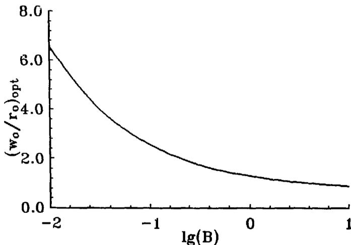
Figure 6: Dependency of the optimal value of the Gaussian beam waist on the beam diffraction parameter
