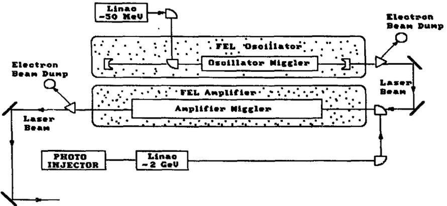
Figure 3: Two-stage FEL scheme for a photon collider
