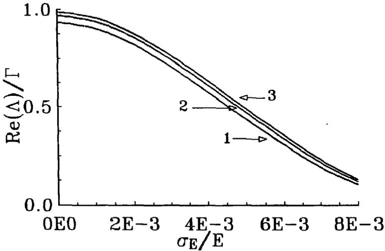
Figure 5: Dependency of the FEL amplifier increment on energy spread: (1) -  $2 \times 0.25$  TeV variant; (2) -  $2 \times 0.5$  TeV variant; (3) -  $2 \times 1$  TeV variant
