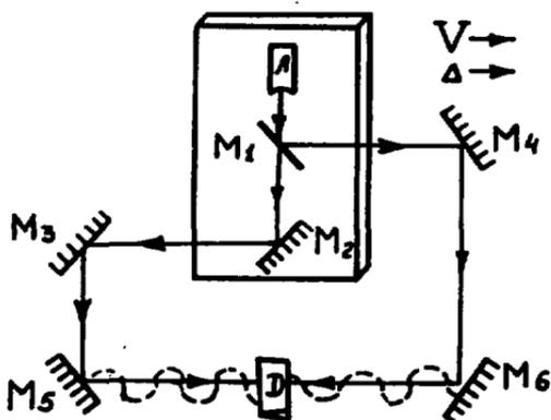
Fig.3. Set-up of the Silvertoothes optical device.
