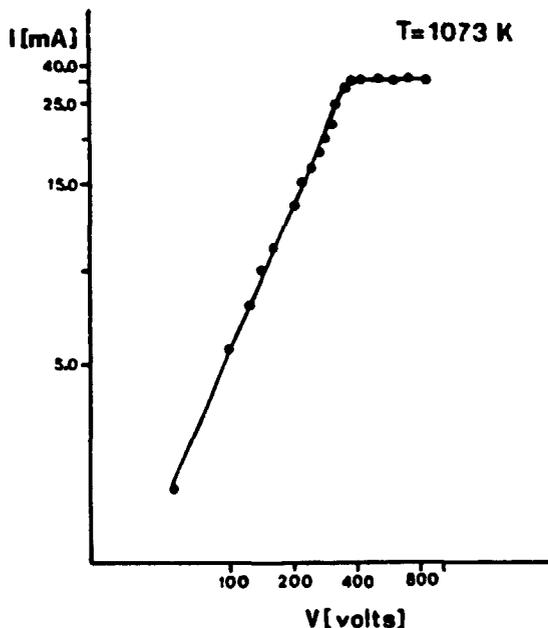
Figure 3. Current-voltage characteristics plotted as  $\ln i$  versus  $V$  at constant cathode temperature
