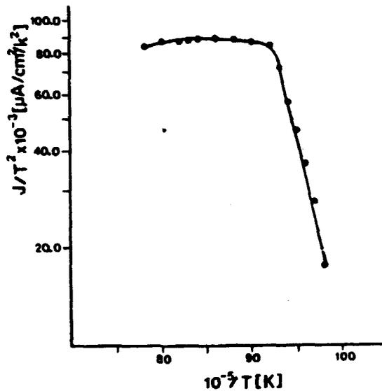
Figure 5. Richardson plot for experimental data
