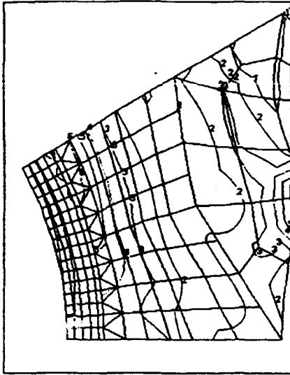
Stress analysis in tube-tubesheet joint
