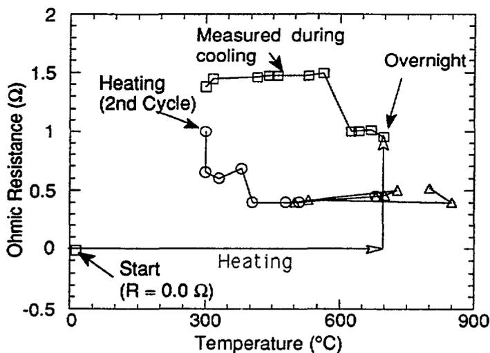
Figure 5. Ohmic resistance vs. temperature during heating cycles.
