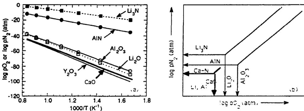
Figure 15. (a) Calculated equilibrium partial pressures of O<sub>2</sub> and N<sub>2</sub> in Li–Al–Y system and (b) schematic thermochemical diagram for M–N–O system, where M represents Al or Li
