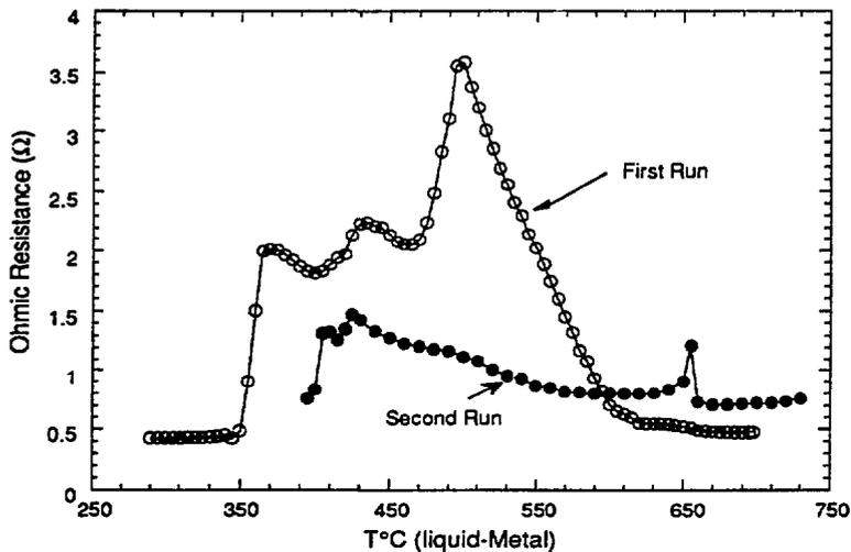
Figure 14. Ohmic values vs. liquid-Li temperature with cooling direction for the two different runs for the in-CaO layer in the V-5Cr-5Ti.
