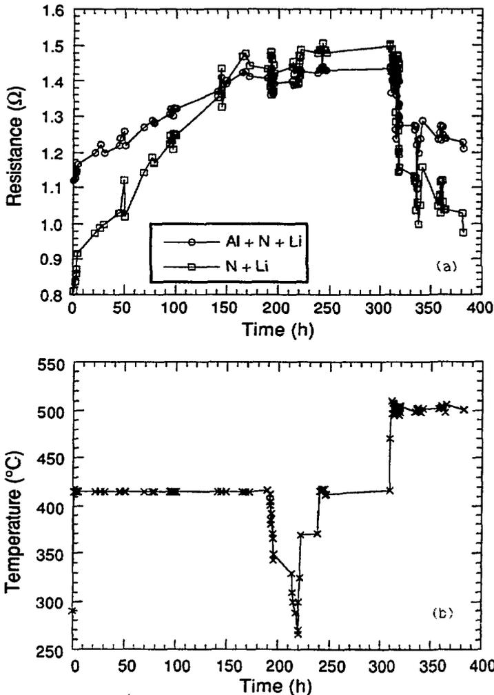
Figure 9. (a) Electrical resistance of V-5%Cr-5%Ti in Li containing N and Al (Cell A) and N (Cell B) and (b) temperature versus time of exposure in the liquid Li environments
