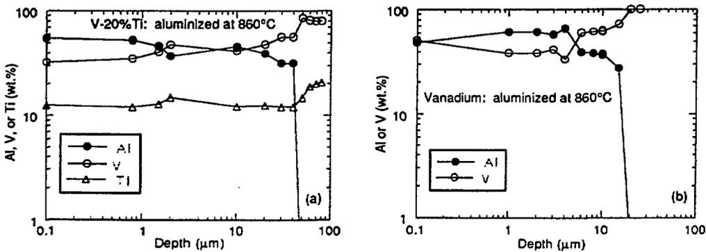
Figure 3. Chemical composition as a function of depth for aluminide layers on (a) V-20%Ti and (b) V
