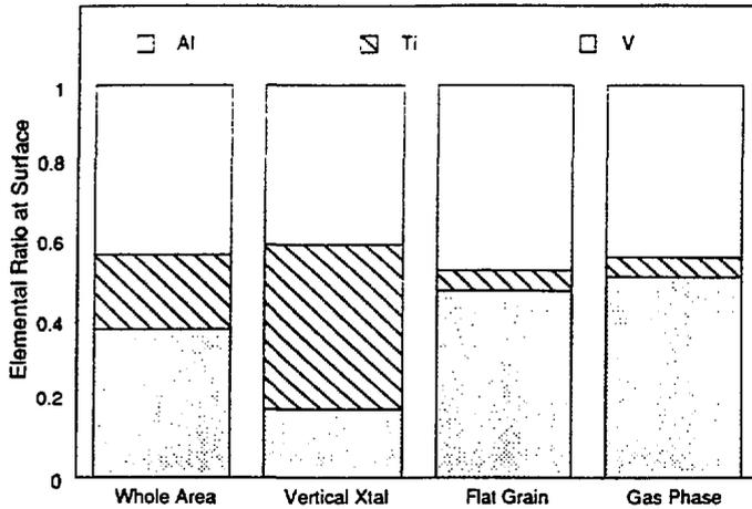
Fig. 8. Element ratio for the exposed (in liquid-Li) and unexposed (in Ar with vapor-Li: gas phase) aluminide coating on V-5%Cr-5%Ti surface.
