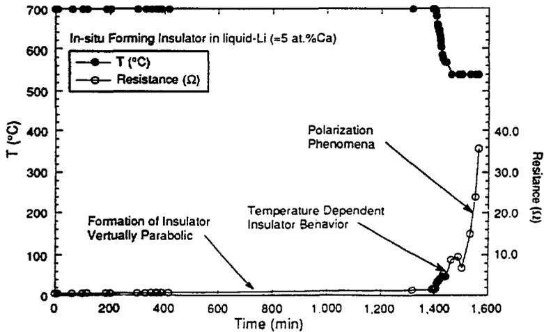
Figure 13. In-situ electrical resistance and liquid-Li temperature measurements as a function of time during fabrication of CaO coating in liquid-Li.
