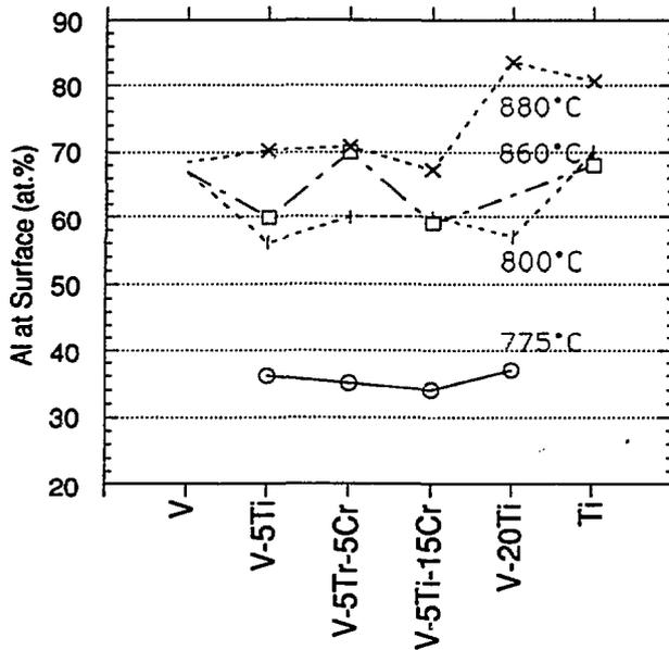
Figure 2. Aluminum content of aluminized surfaces formed on several V-base alloys and Ti at several temperatures between  $775$  and  $880^\circ\text{C}$
