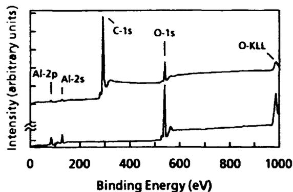
Fig. 1 XPS survey scans of (upper) as synthesized powder and (lower) 1200°C heat treated powder. The atomic Al/O ratios, as determined by quantitative XPS analysis, are 0.52 and 0.67 respectively (theoretical value: Al/O = 0.66).
