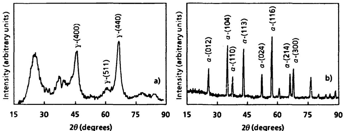
Fig. 2 X-ray  $\text{CuK}\alpha$  diffraction pattern recorded in reflexion geometry: a) as synthesized powder; b) after thermal treatment at 1200°C.
