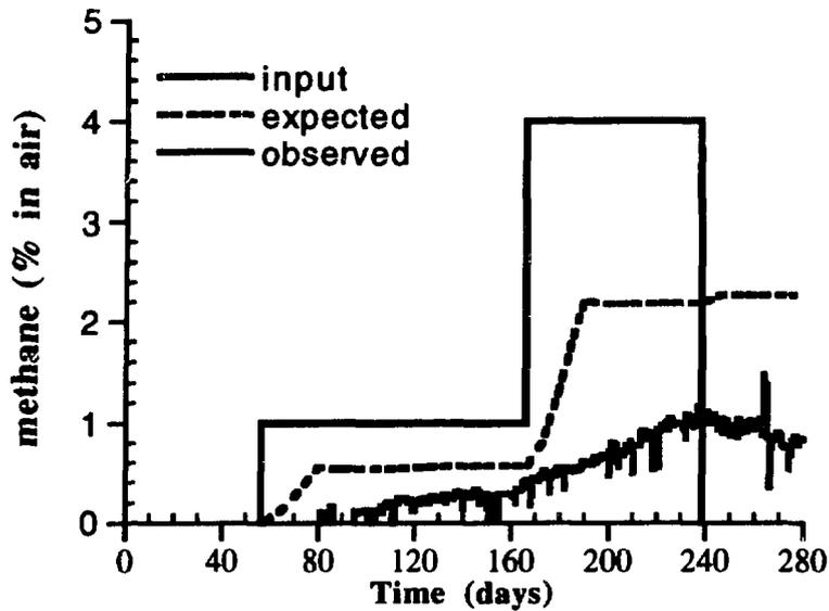
Fig. 4.12. Methane injected and methane at the extraction well vs. time (expected and observed). The expected methane levels are projections based on a helium tracer test.
