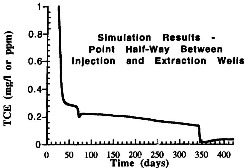
Fig. 4.20. Simulated TCE concentration vs. time profile at point half-way between injection and extraction wells.
