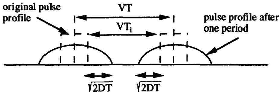
Fig. 5.1. Schematic illustrating separation of pulses and diffusion of original square wave pulses.
