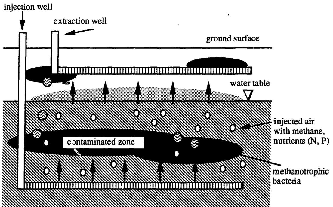
Fig. 2.3. Schematic of *in situ* bioremediation technology.
