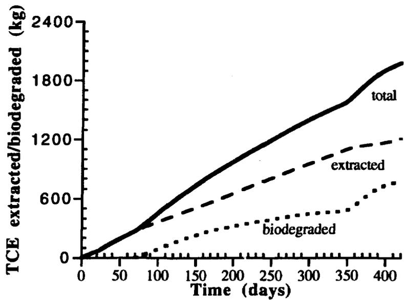
Fig. 4.11. TCE extracted/degraded vs. time for *in situ* bioremediation simulation.
