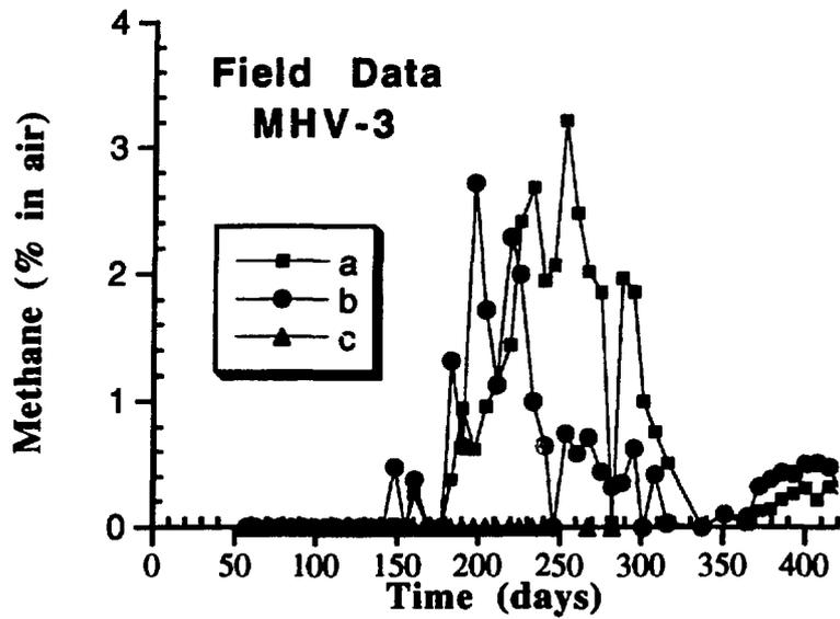
Fig. 4.16. Observed methane concentration vs. time profile at MHV-3. Data from Hazen (1992b).
