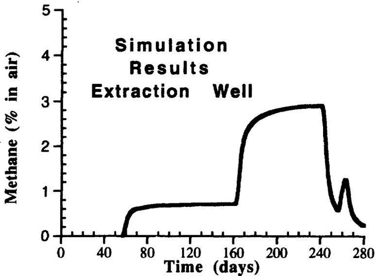
Fig. 4.13. Simulated methane concentration vs. time profile at the extraction well.
