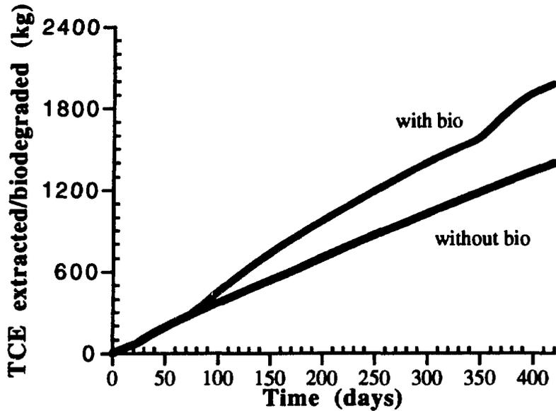
Fig. 5.4. TCE extracted/degraded vs. time for *in situ* bioremediation simulation and an identical simulation without microbial activity.
