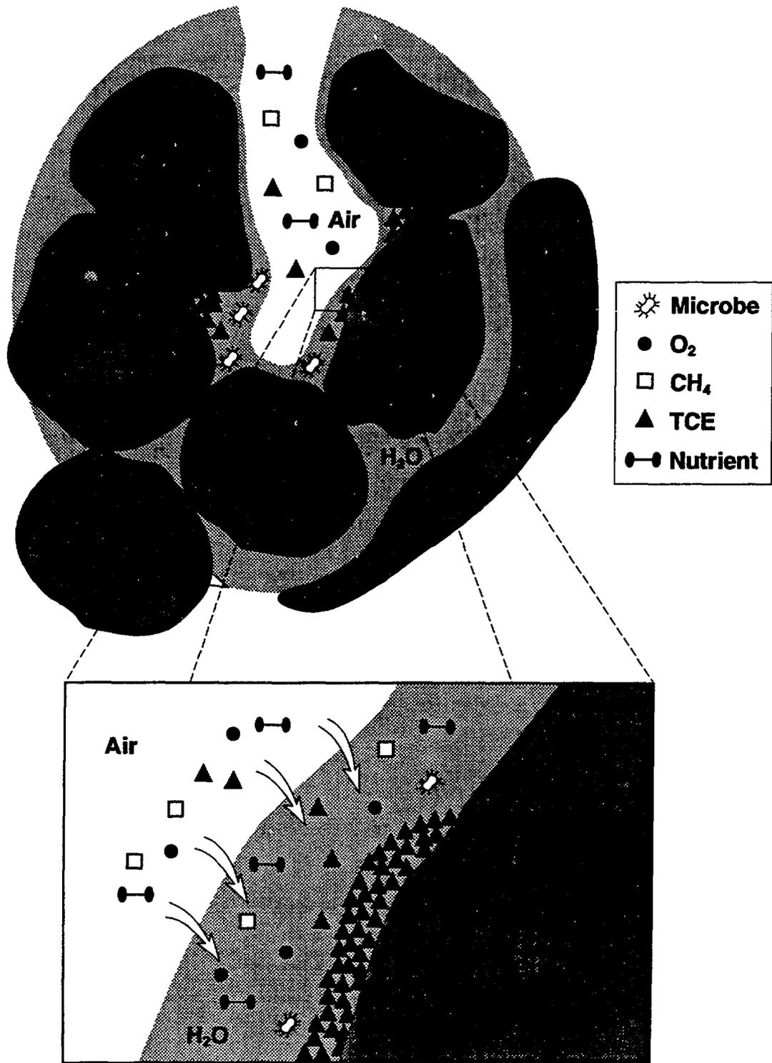
Fig. 2.4. Schematic illustration of bioremediation processes at the pore-scale.
