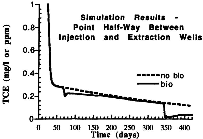
Fig. 5.5. Simulated TCE concentration vs. time profiles at a point half-way between injection and extraction wells for simulations with and without microbial activity.
