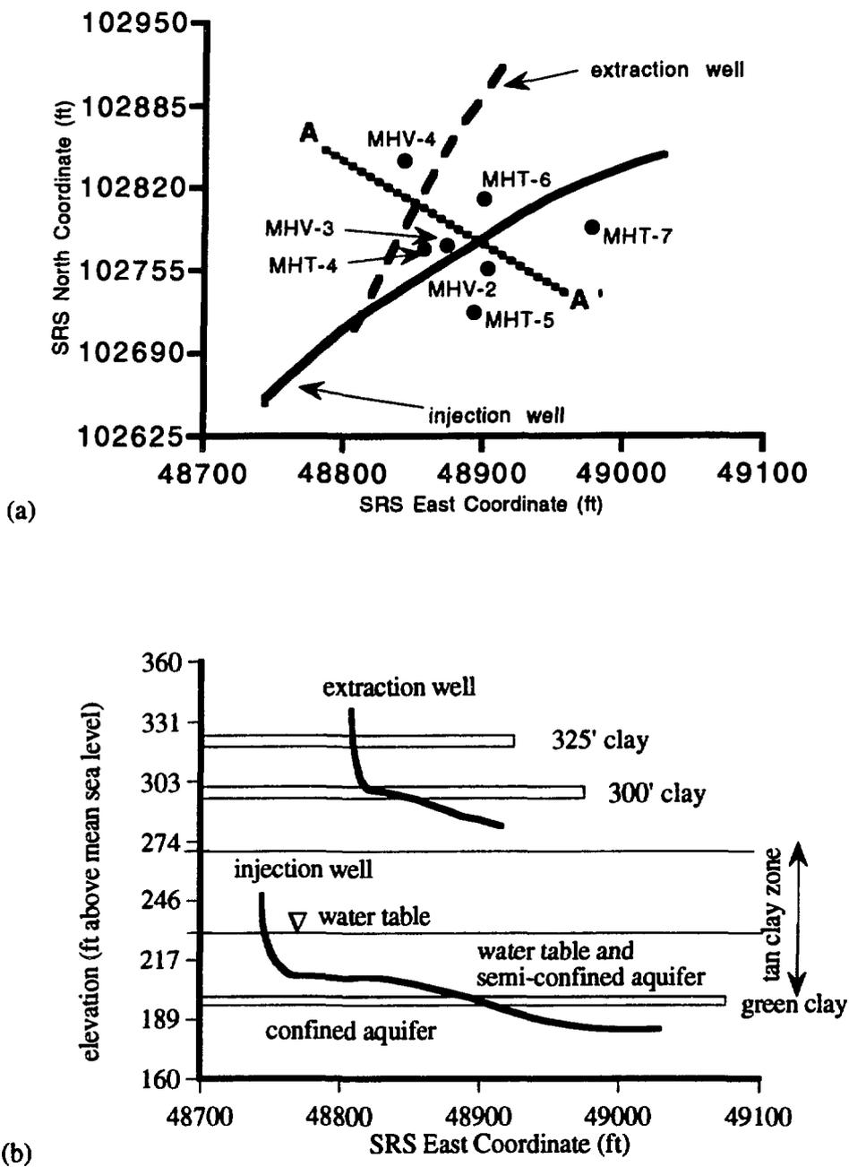
Fig. 2.2. Generalized hydrogeology and location of horizontal wells (a) map view, (b) cross-section. A-A' represents the 2-D cross-section modeled in our simulations.
