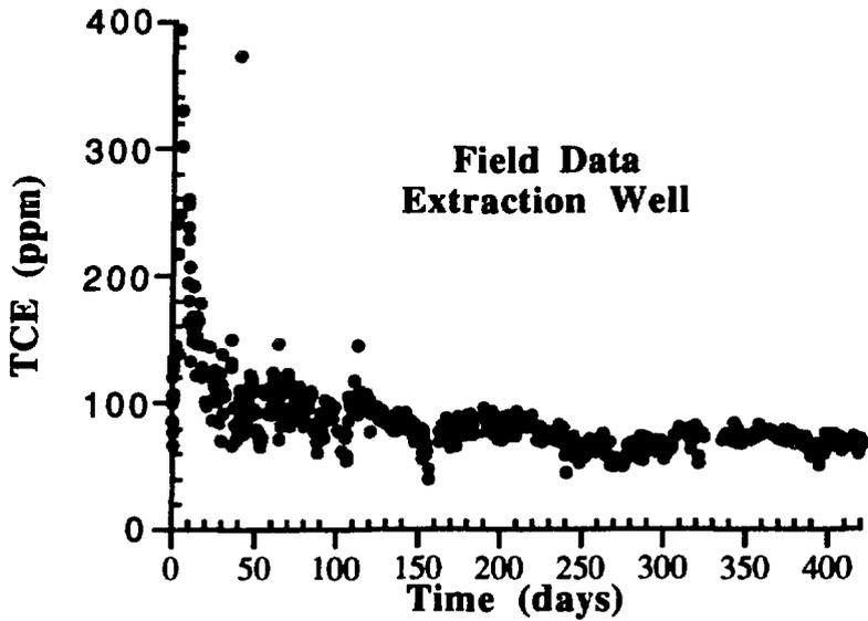
Fig. 4.14. Observed TCE concentration vs. time profile at the extraction well. Data from Hazen (1992b).
