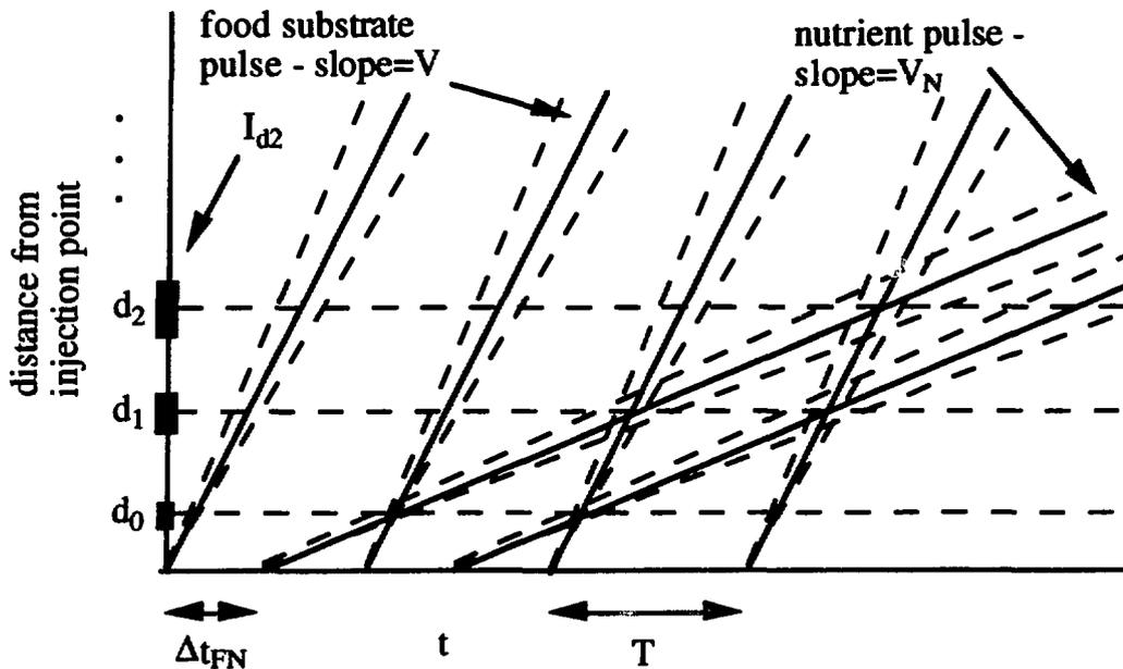
Fig. 5.2. Plot of food substrate pulse and nutrient pulse as a function of distance and time. Enhanced microbial growth and biodegradation will occur at the intersections of the nutrient (slope =  $V_N$  lines) and the food substrate pulses (slope =  $V$  lines) ( $V_N < V$  case.)
