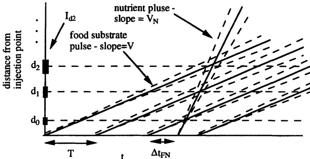
Fig. 5.3. Plot of food substrate pulse and nutrient pulse as a function of distance and time. Enhanced microbial growth and biodegradation will occur at the intersections of the nutrient (slope =  $V_N$  lines) and the food substrate pulses (slope =  $V$  lines) ( $V < V_N$  case.)
