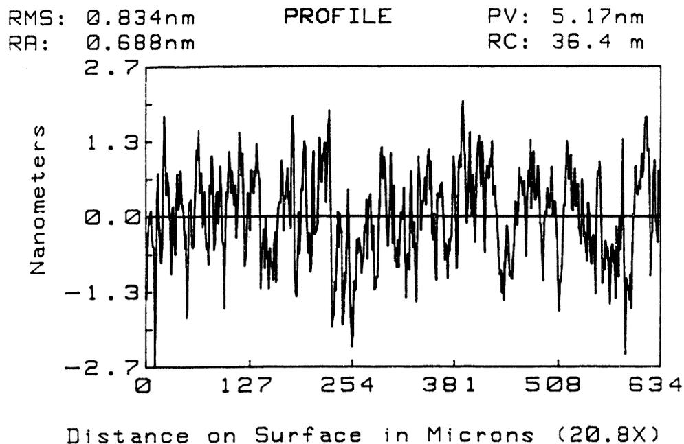
Figure 5. Surface scan of a diamond turned cerium fluoride sample. The surface finish is measured to be 8 Å RMS.
