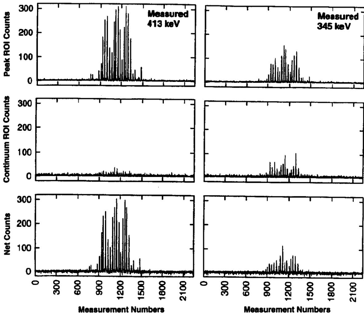
*Fig. 3. Experimental TGS data for a medium density, low-Z matrix ( $0.6 \text{ g/cm}^3$  polyethylene beads) containing 3 g of high-burnup plutonium. Each measurement number uniquely corresponds to a scan-position (angle, displacement, elevation) determined by the scanning protocol.[2]*
