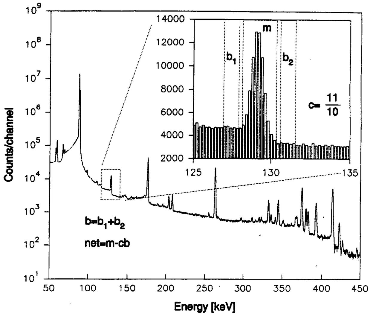
Fig. 1. An HRGS spectrum for a high-burnup plutonium source in a 55-gal. drum containing a medium-density matrix. Symmetric ROIs for continuum subtraction are shown in the exploded view for the 129-keV gamma ray emitted by  $^{239}\text{Pu}$ .
