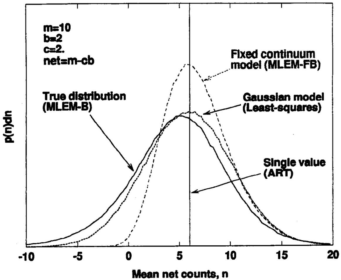
Fig. 6. The distribution of mean net counts for several models of the statistical structure of the full-energy measurements.
