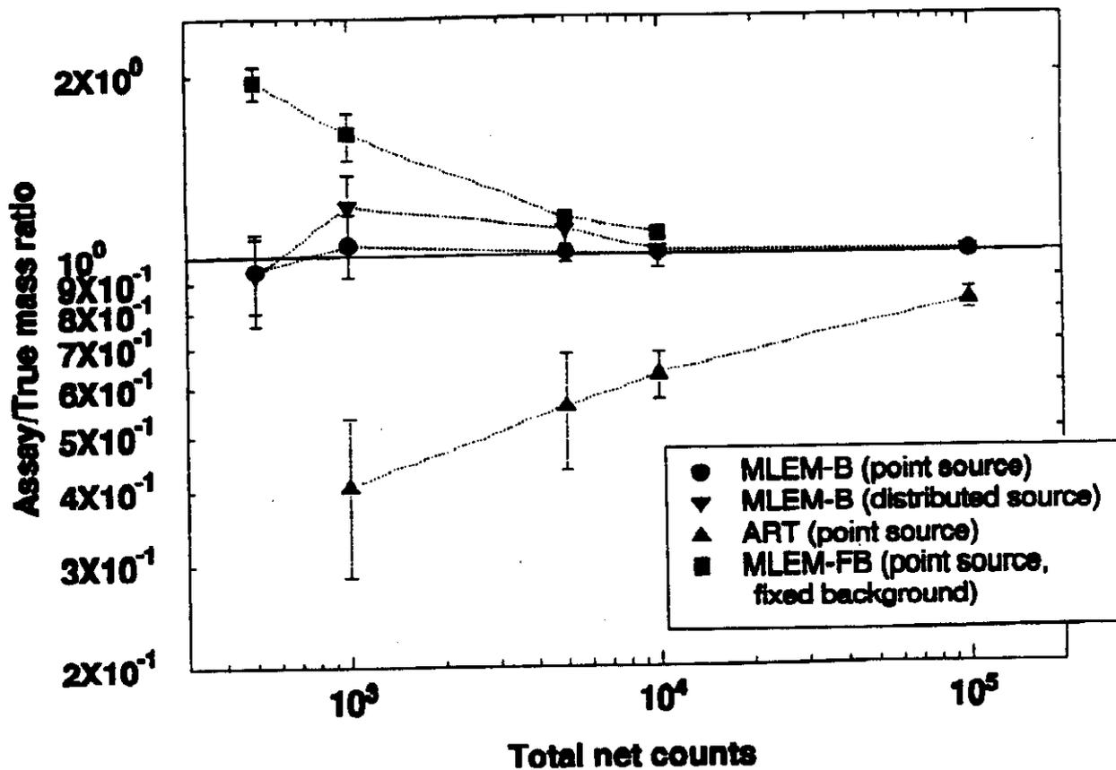
Fig. 5. Bias for various reconstruction algorithms as a function of total net counts for a fixed continuum level of 80%.
