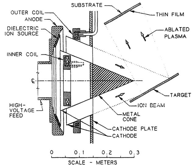
Fig. 2 Ion diode configuration used in HIPBD
