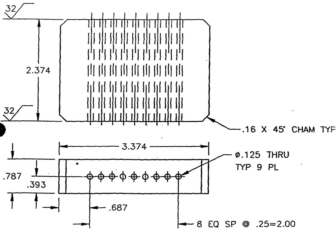
Figure 5 Schematic of a 9-hole cryogenic crystal used to test the liquid nitrogen pumping system performance
