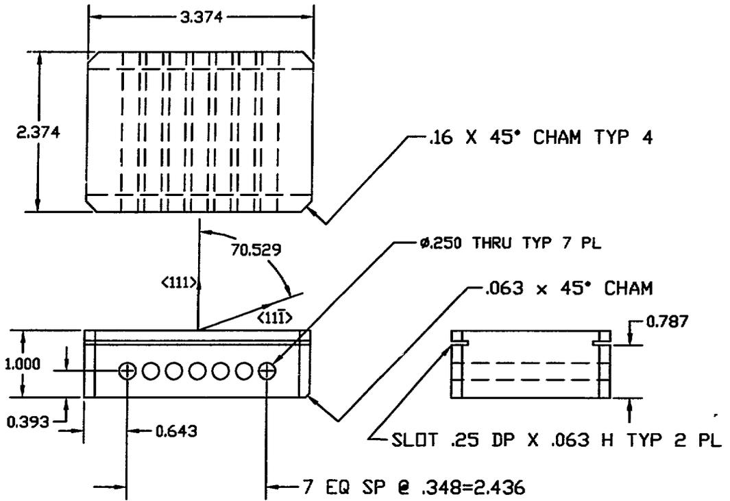
Figure 9 Schematic of cryogenic crystal for use with Cu mesh inserts
