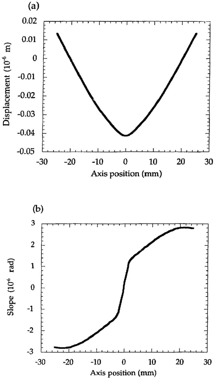
Figure 7 (a) Displacement, and (b) slope of crystal surface along the central axis from finite element analysis of inclined crystal for Undulator A
