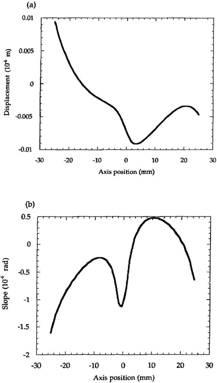
Figure 8 (a) Displacement, and (b) slope of diffraction plane along the central axis from finite element analysis of inclined crystal for Undulator A
