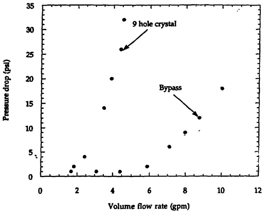
Figure 4 Liquid nitrogen pumping system performance for flow through bypass and a 9-hole crystal
