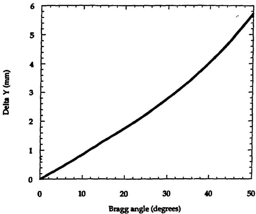
Figure 2 Vertical walk of beam at 10 meters from the monochromator with first crystal at 100 K and the second crystal at 293 K.
