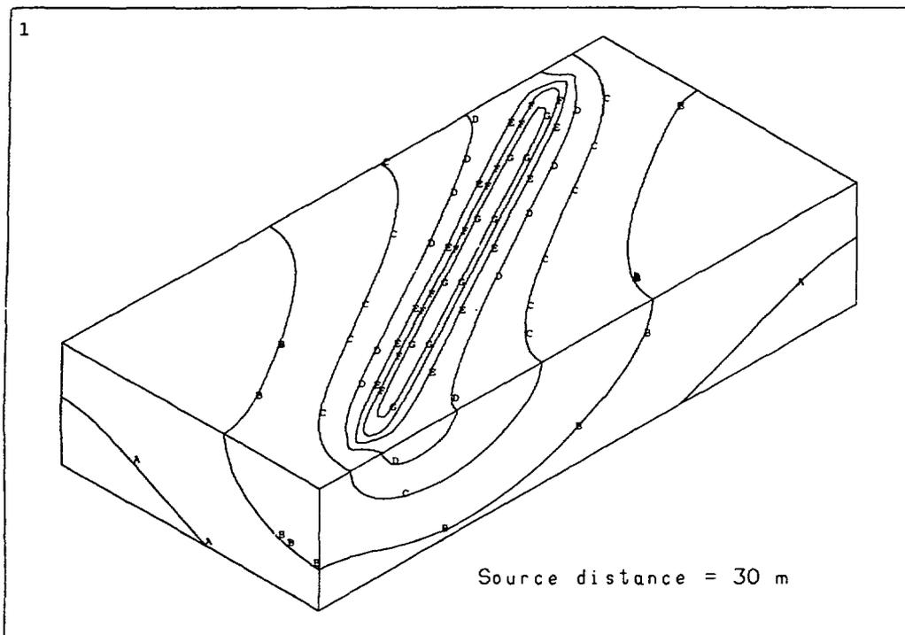
Figure 6 Thermal results from finite element analysis for 80° inclined cryogenic crystal for Undulator A
