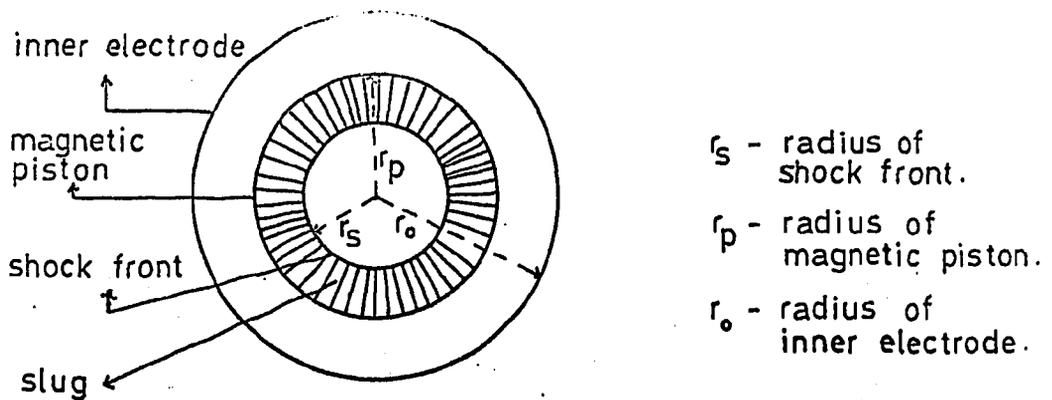
Figure (2) Cross-section of the radial compression .
