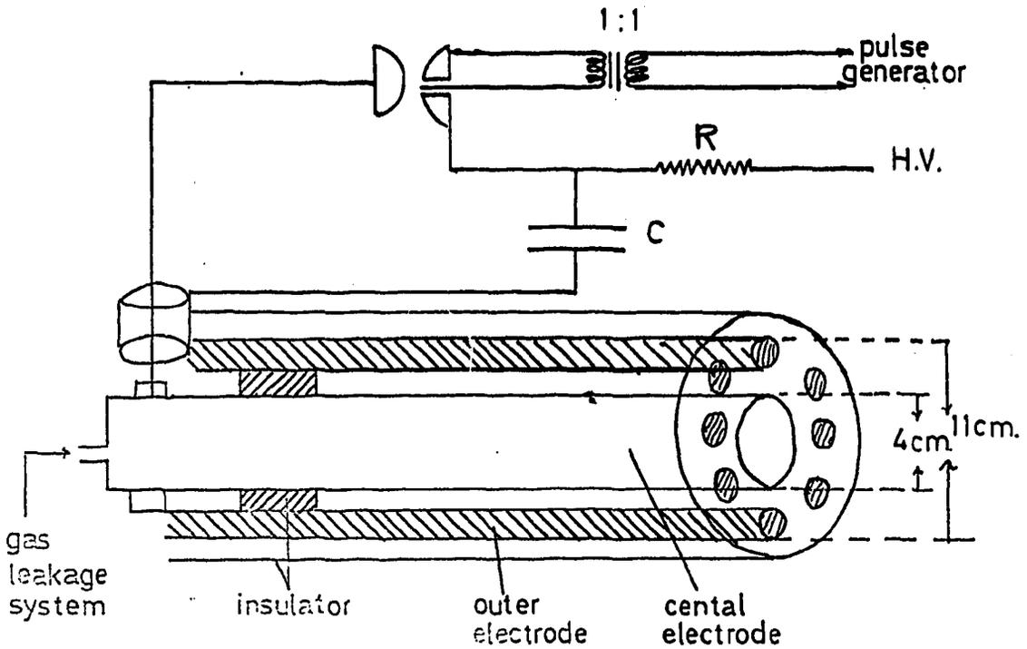
Figure (1) Schematic diagram of plasma focus device.
