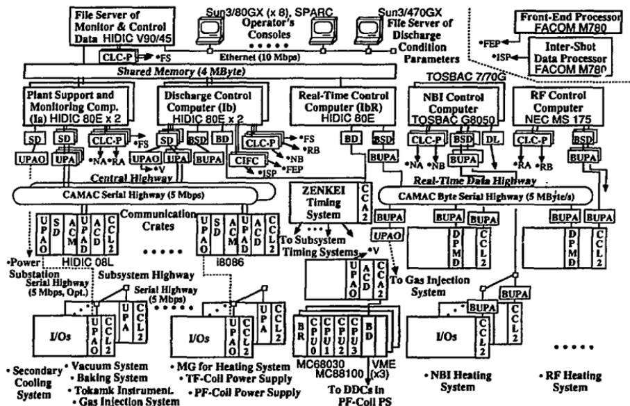
Fig. 1 Computer Configuration of the JT-60 Control System
