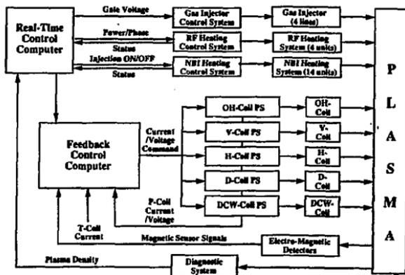
Fig. 2 Data flow of the JT-60U plasma control system
