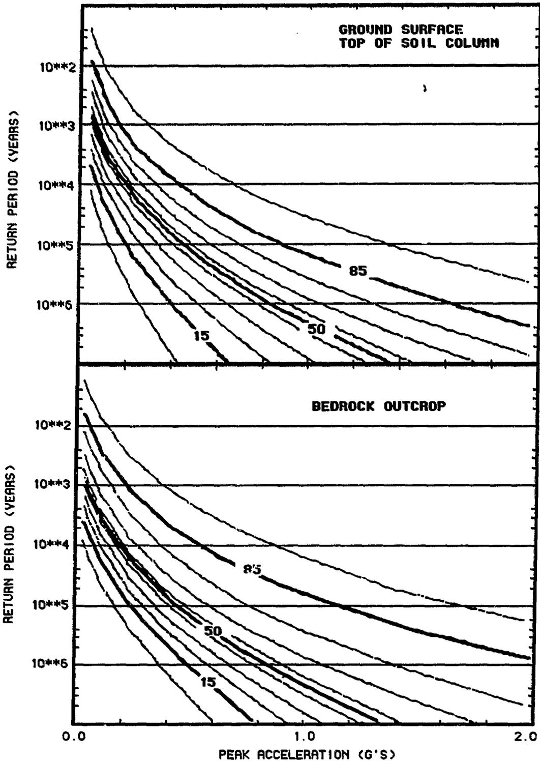
**FIGURE 5 BEDROCK AND SURFACE HAZARD PREDICTION FOR HFBR SITE FROM LLNL USING 5 GM EXPERTS**
