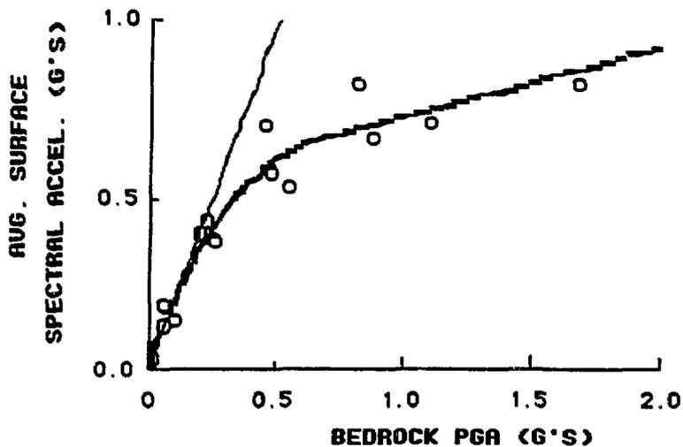
**FIGURE 7 COMPUTED CONVERSION OF BEDROCK PGA TO SURFACE AVERAGE (5 TO 10 HZ) SPECTRAL ACCELERATION**
