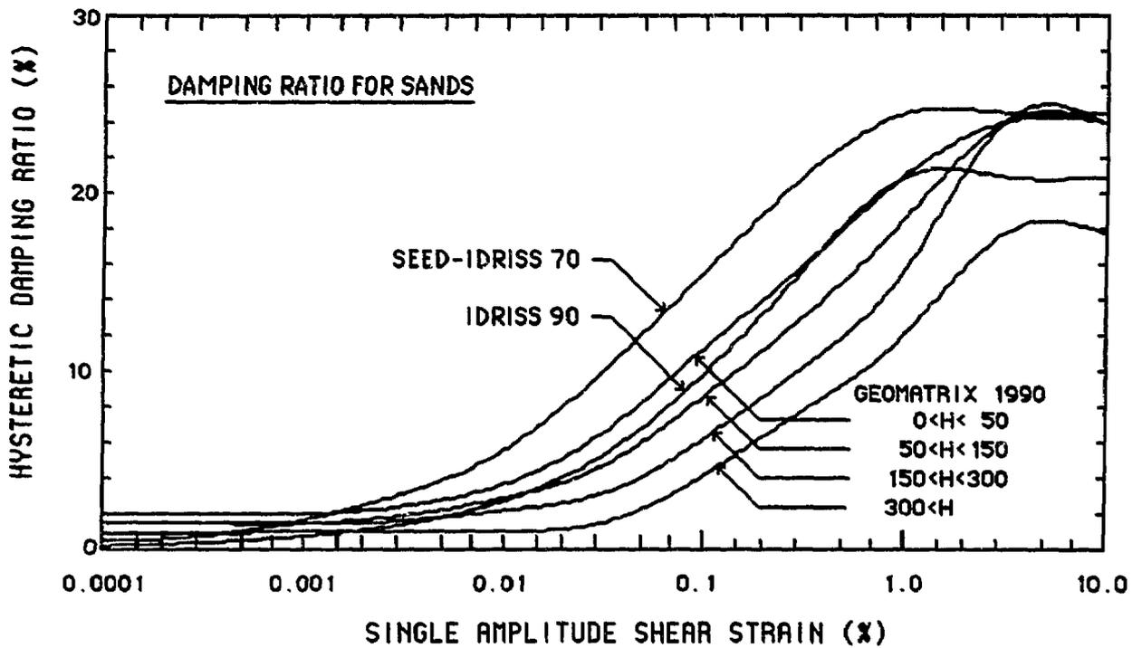
**FIGURE 3 SHEAR DEGRADATION MODELS FOR SANDS**
