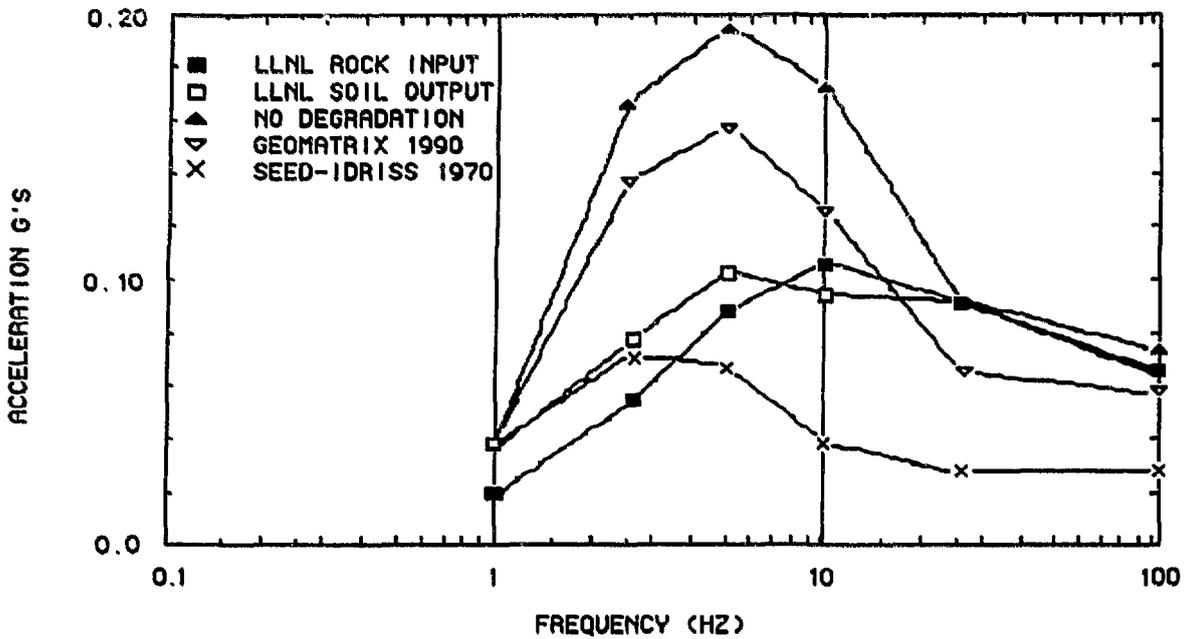
**FIGURE 6 COMPUTED MEDIAN SURFACE SPECTRA FOR 1000 YEAR RETURN PERIOD AND 50TH PERCENTILE ROCK OUTCROP MOTION**
