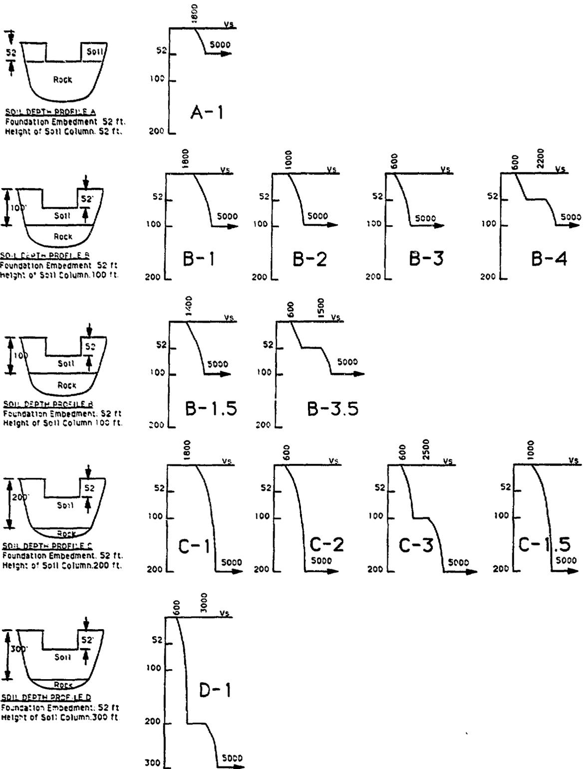
**Figure 3 - Generic Soil Profiles for Soil and SSI Analysis**
