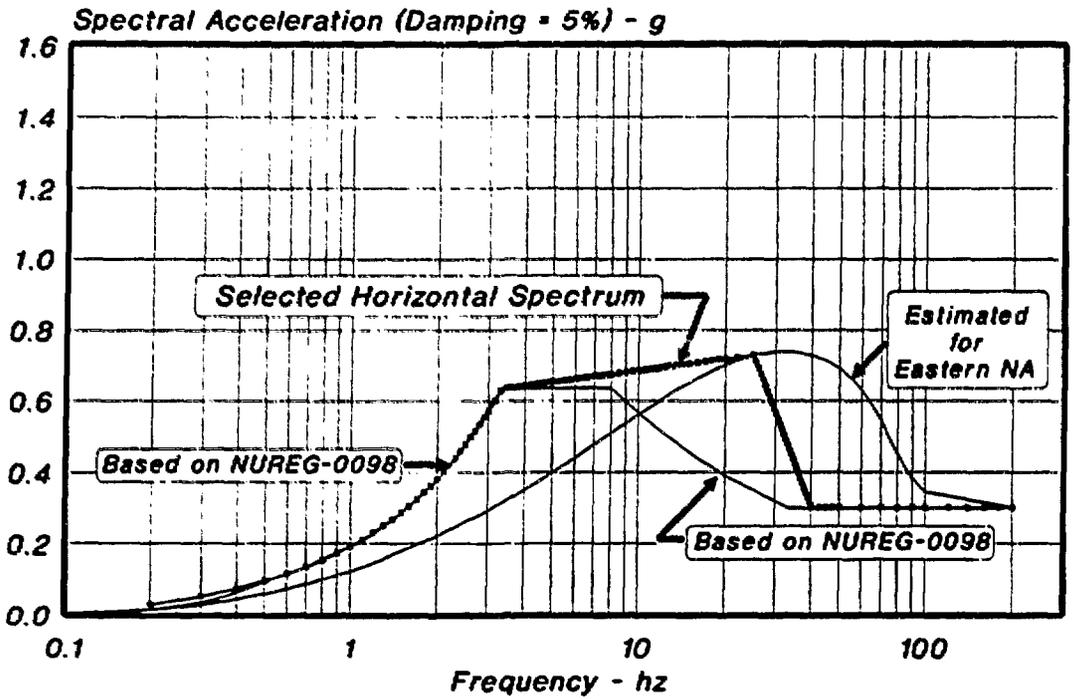
**Figure 2 - Selected Design Response Spectrum at Rock Outcrop**
