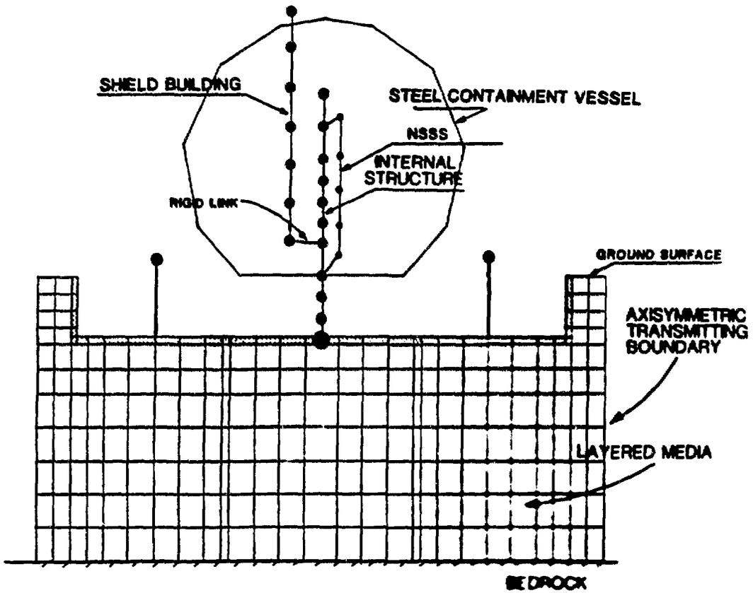
**Figure 4 - Schematic Representation of the Combined Structural Model of the Power Generation Complex Used in the Reactor Building Analysis**
