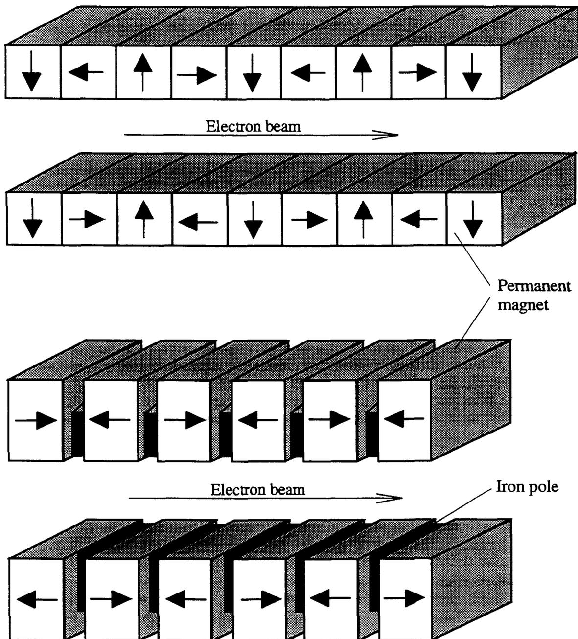
Fig. 5 Magnet configurations for planar insertion devices. The pure magnet configuration (top) employs eight magnet blocks per field period while the hybrid configuration (bottom) has four poles and four magnet blocks.
