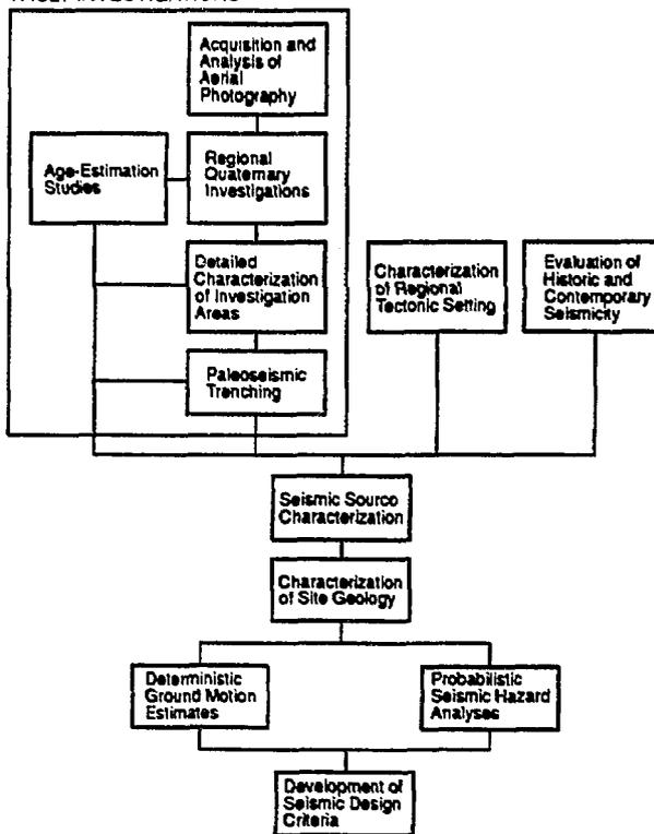
Figure 3. FLOW DIAGRAM OF LANL SEISMIC HAZARD STUDIES.
