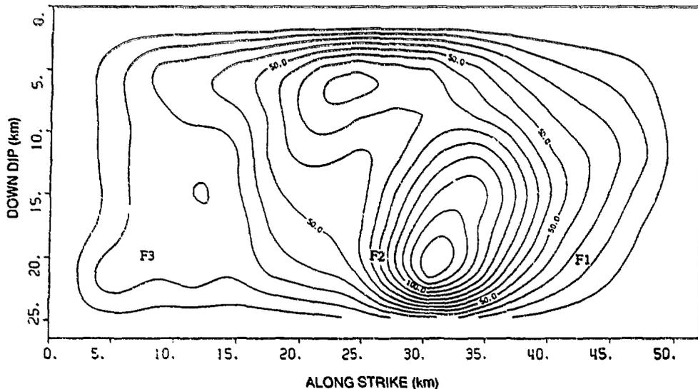
Figure 4. 1983 BORAH PEAK EARTHQUAKE SLIP DISTRIBUTION [19] USED IN FINITE FAULT MODELING FOR THE SOUTHERN LEMHI FAULT EARTHQUAKE. SLIP IS IN CM.
