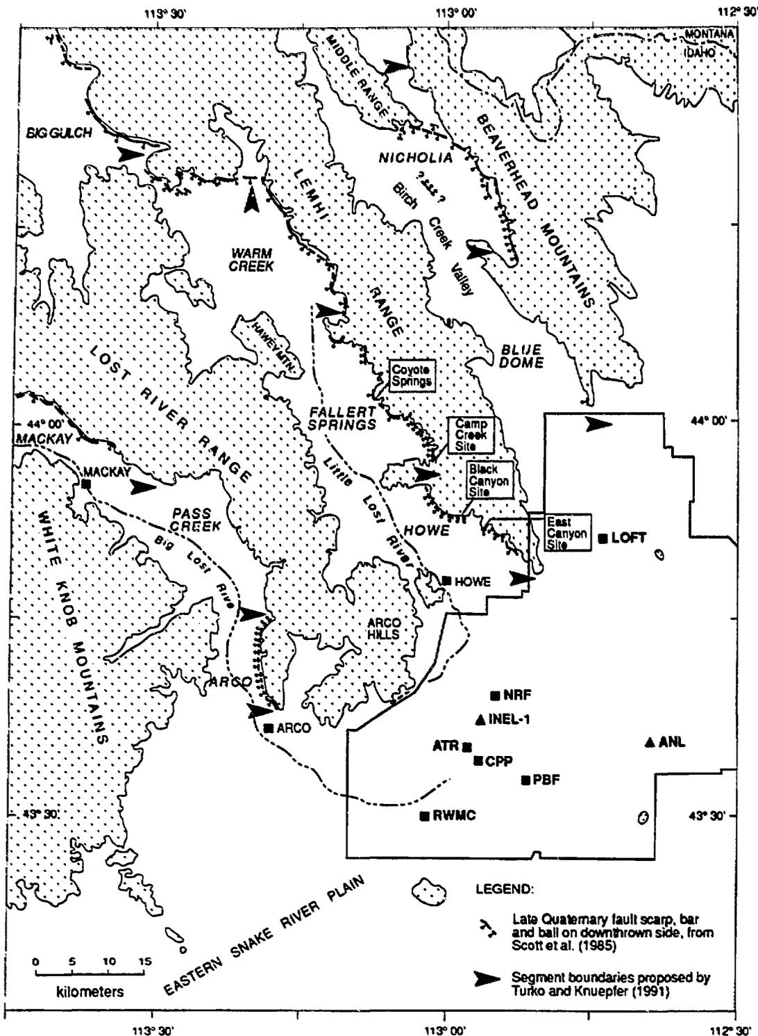
Figure 1. LOST RIVER, LEMHI AND BEAVERHEAD FAULTS ADJACENT TO THE INEL. ALSO SHOWN ARE PALEOSEISMIC TRENCH SITES INVESTIGATED ALONG THE SOUTHERN LEMHI FAULT [1, 2].
