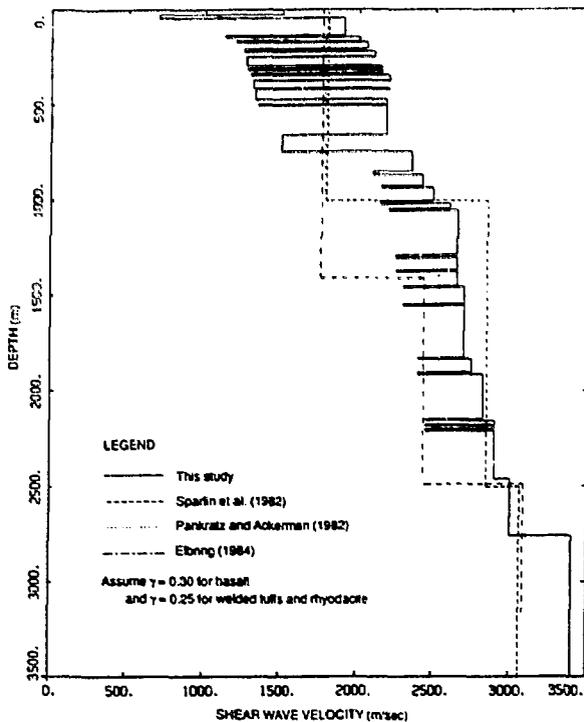
Figure 3. SHEAR-WAVE VELOCITY PROFILE AT THE INEL-1 DRILLHOLE.
