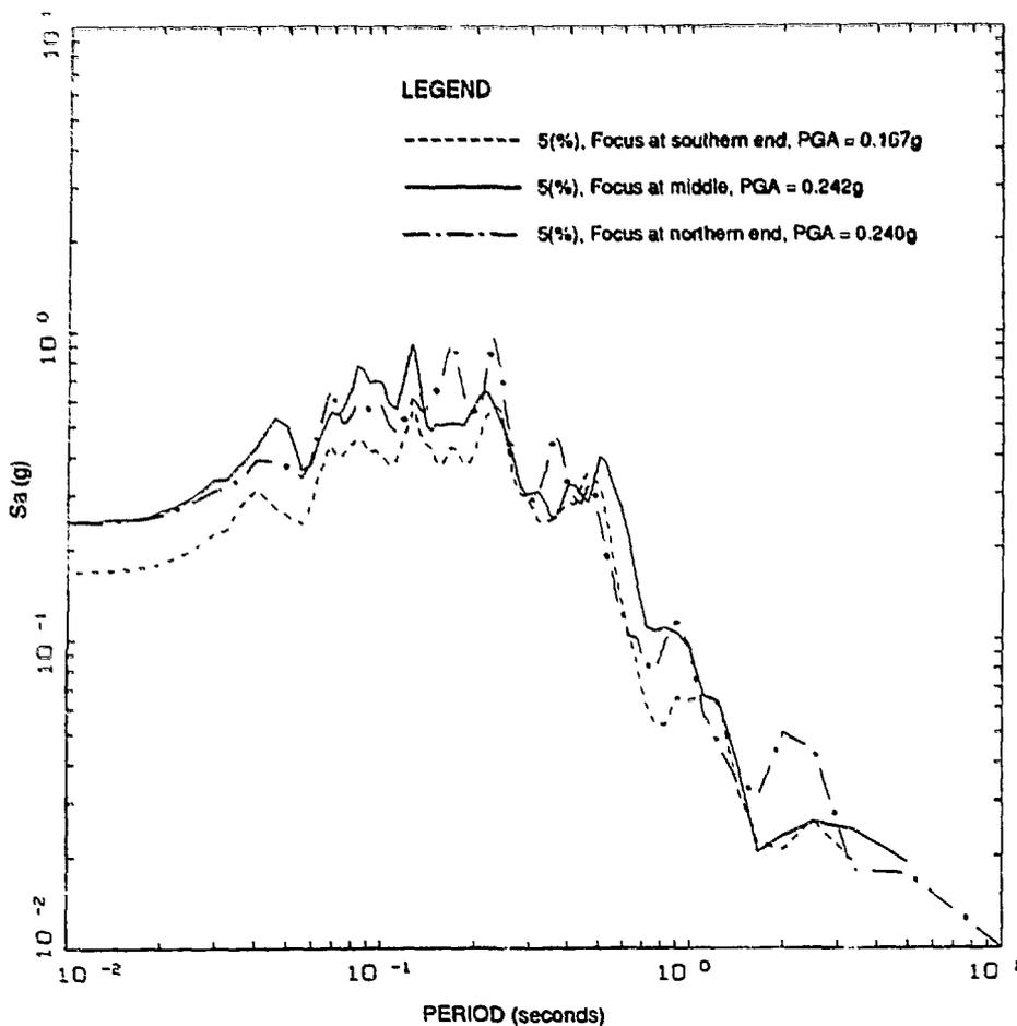
Figure 5. ACCELERATION RESPONSE SPECTRA FROM FINITE FAULT MODELING.
