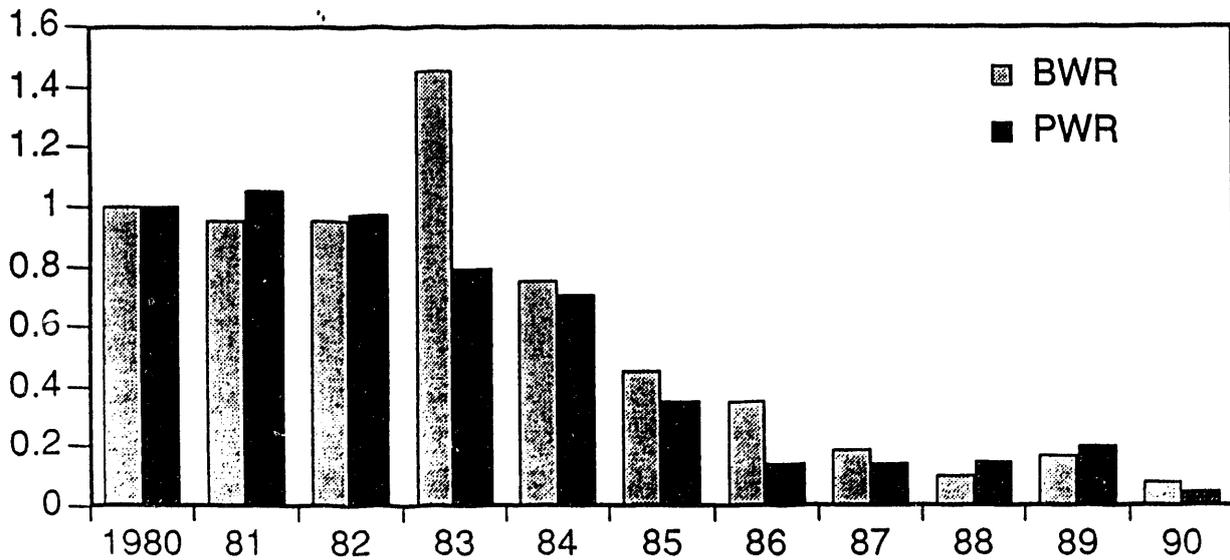
Figure 3. (Volume X Activity) of PWR and BWR LLW shipped annually from 1980 to 1990, per MW(e) normalized to 1980 values (ref. 4)
