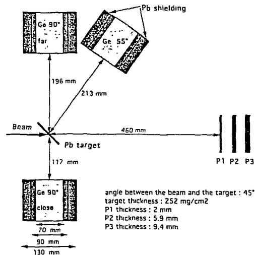
Figure 8 : Experimental set-up.
