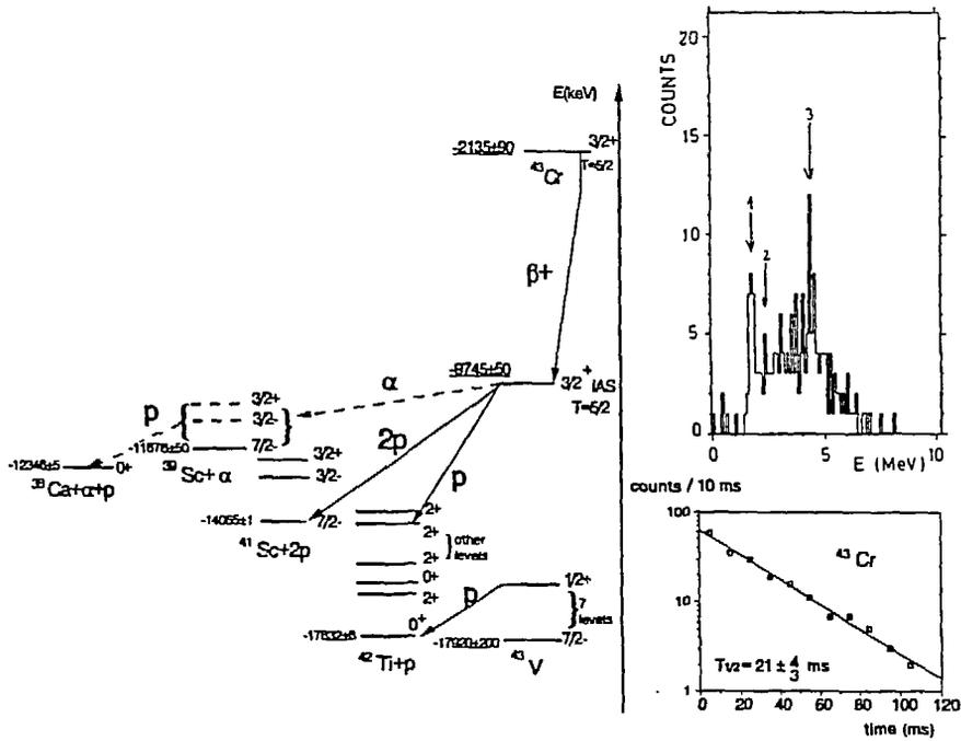
Figure 3. : Partial decay scheme proposed for  $^{43}\text{Cr}$ . Each state is labelled with its mass-excess energy. The mass-excess values derived in the present work are underlined. The spin and parity, if known, are indicated ; otherwise, the spin and parity of the corresponding level in the mirror nuclei are adopted.
