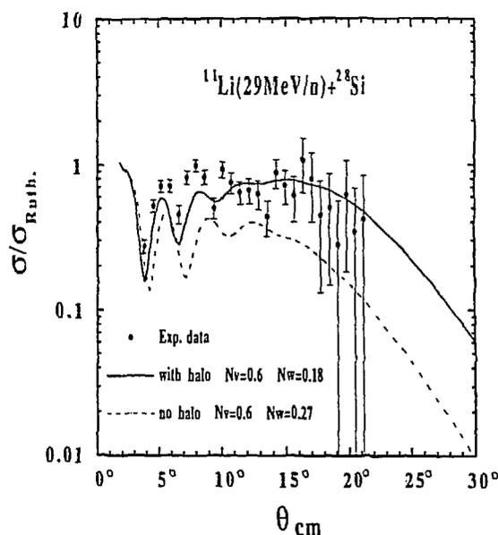
Figure 5. : Measured angular distribution and coupled-channel calculation for the elastic scattering of 29 MeV/u  $^{11}\text{Li}$  on a silicon target <sup>9</sup>.
