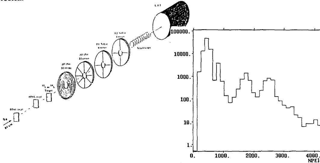
Fig.6. : This set-up is designed for the study of  ${}^8\text{B}$  elastic scattering. The break-up reaction  ${}^8\text{B} \rightarrow {}^7\text{Be} + p$  is also measured : the telescope of eleven 300  $\mu\text{m}$  thick silicon detectors selects the  ${}^7\text{Be}$  nuclei produced in the reaction. The insert shows a very preliminary angular distribution measured for the scattered  ${}^8\text{B}$  nuclei.
