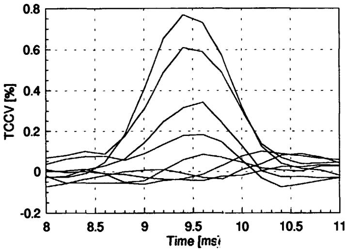
Figure 8: Triple cross-covariance for beams crossing in inner tube.
