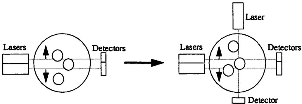
Figure 3: Geometries for axial and radial correlation length determination.
