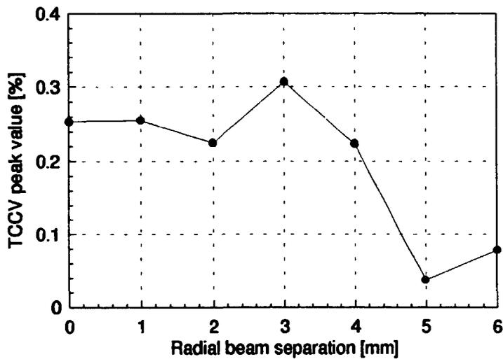
*Figure 13: Absolute value of radial cross-covariance in water-air flow experiment.*
