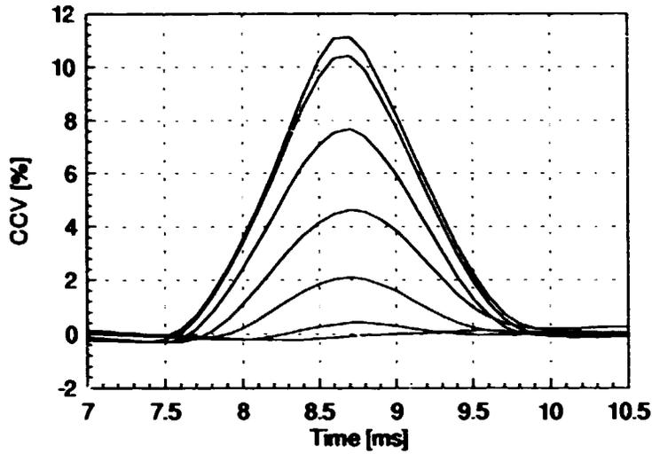
*Figure 5: Cross-covariance for radially shifted, parallel beams and 3 mm glass beads.*
