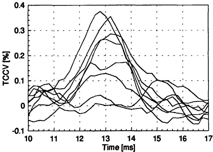
Figure 9: Triple cross-covariance for beams crossing in outer tube.
