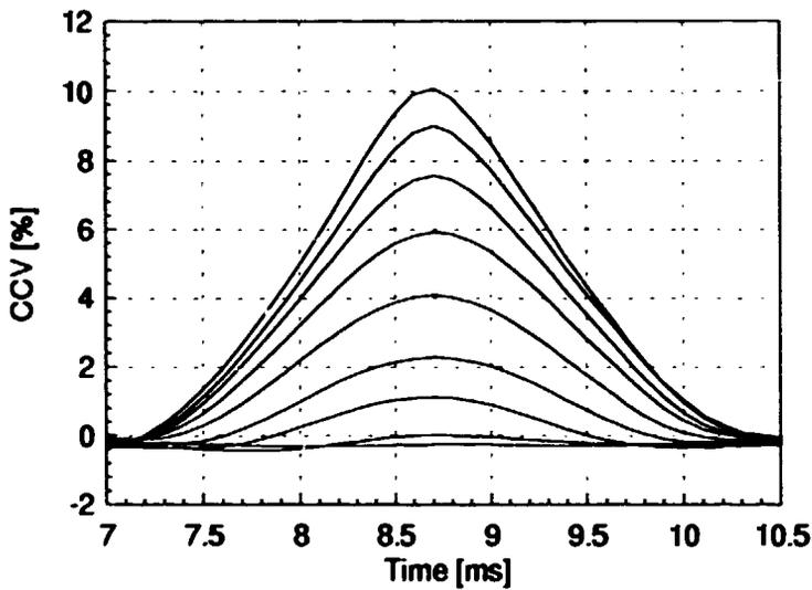
*Figure 6: Cross-covariance for radially shifted, parallel beams and 4 mm glass beads.*
