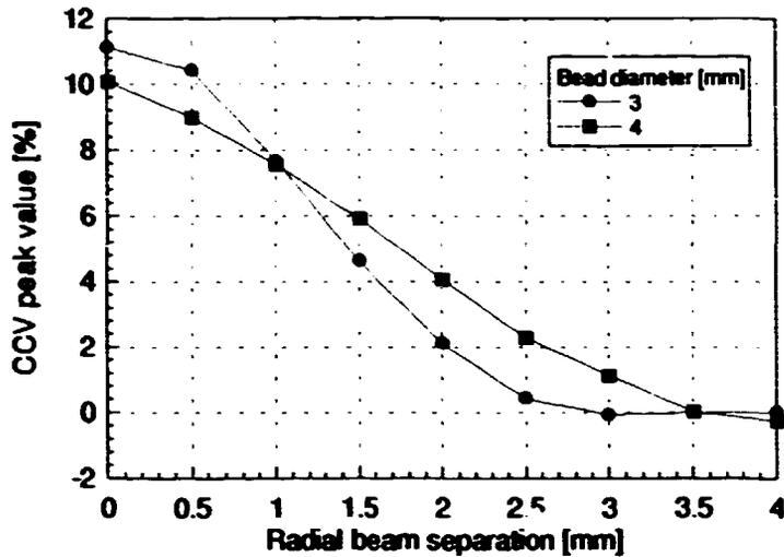
Figure 7: Radial cross-covariance for different bead sizes.
