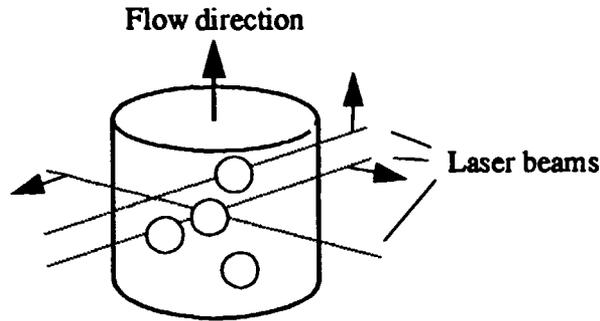
Figure 4: Geometrical arrangement of laser beams.
