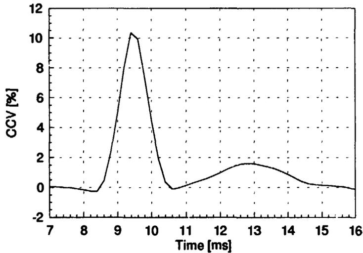
Figure 11: Cross-covariance from two, parallel beams.
