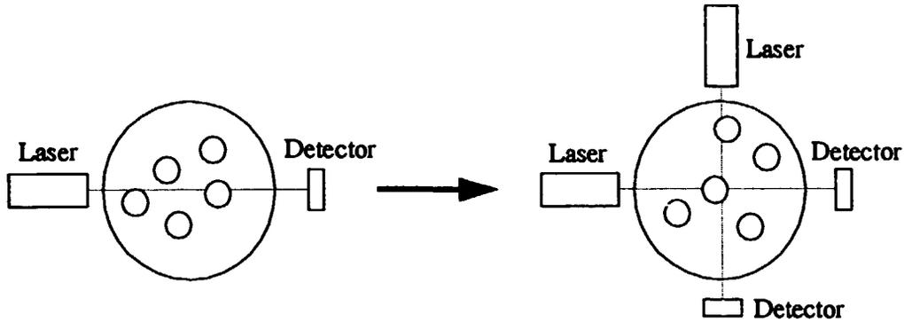
Figure 2: Geometries for axial correlation length determination.
