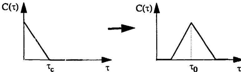
Figure 1: Autocovariance from one beam and cross-covariance from two, parallel and axially shifted beams.
