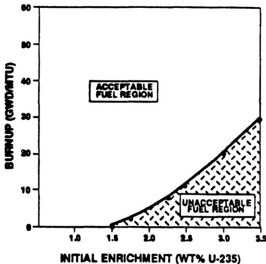
Figure 1. Example Burnup Credit Loading Curve
