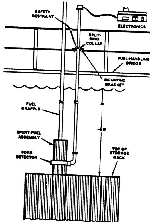
Figure 3. FORK System Arrangement in Spent Fuel Pool
