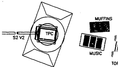
Fig. 1: Detector setup for EOS experiment. The beam enters from the left and the target is located at the entrance to the TPC.
