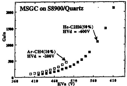
Figure 3: Gas gain dependence on the anode voltage for the MSGC on thin-film Pestov glass on a quartz substrate in two different gas mixtures.
