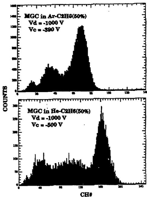
Figure 6:  $^{55}\text{Fe}$  x-ray spectra measured by a MGC (a) in the  $\text{Ar-C}_2\text{H}_6(50\%)$  gas mixture (upper), and (b) in the  $\text{He-C}_2\text{H}_6(50\%)$  gas mixture (lower).
