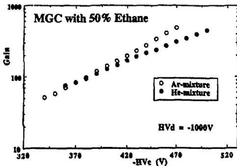
Figure 7: Gas gain dependence on the cathode voltage for a MGC in two different gas mixtures.
