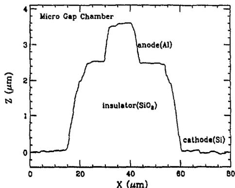
Figure 4: The cross-sectional view of a Micro Gap Chamber.
